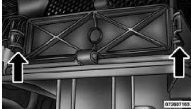
A/C Air Filter Replacement
