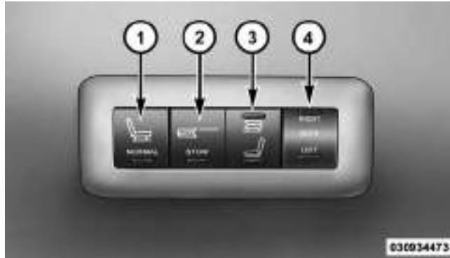
Rear Panel Power Switch Bank
