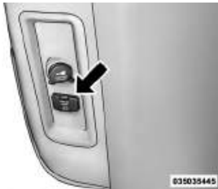
Power Inverter Outlet
