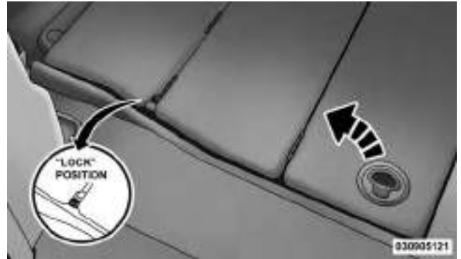
Storage Bin Cover Lock Release
