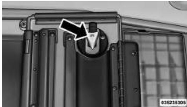
Storage Bin Cover Emergency Release Lever
