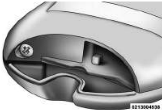
Remove Screw From Transmitter Case
