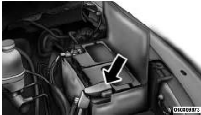
Positive Battery Post
