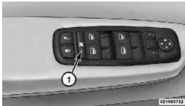
Window Lockout Switch
