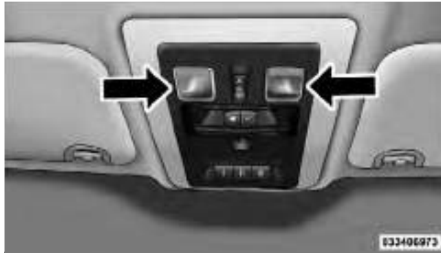
Front Courtesy/Reading Lights
