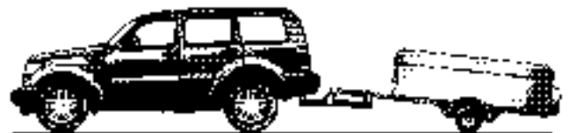
FIG. 3 IMPROPER ADJUSTMENT (INCORRECT)
