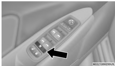
Window Lockout Switch
