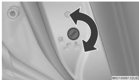
Child-Protection Door Lock Function
