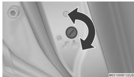
Child-Protection Door Lock Function
