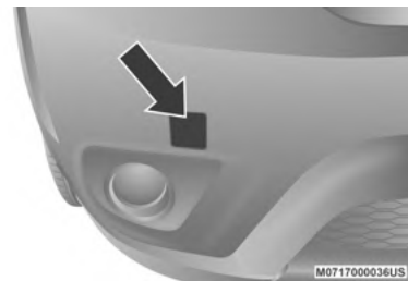
Front Tow Eye Installed
