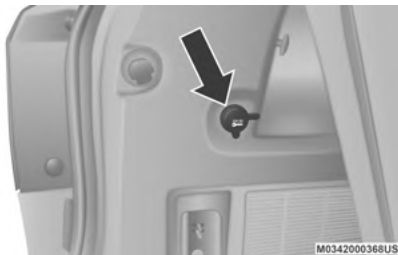
Rear Cargo Area Power Outlet
