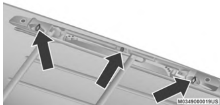
Rail Tie Loops
