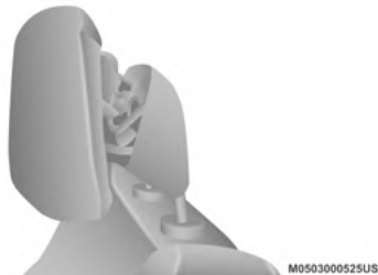
Active Head Restraint (AHR) Deployed
