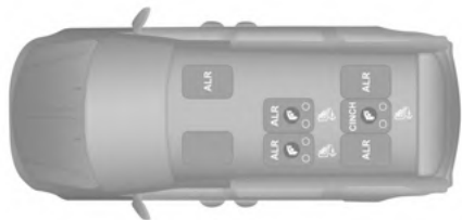
ALR – Switchable Automatic Locking Retractor (2nd Row Bench Seat )
