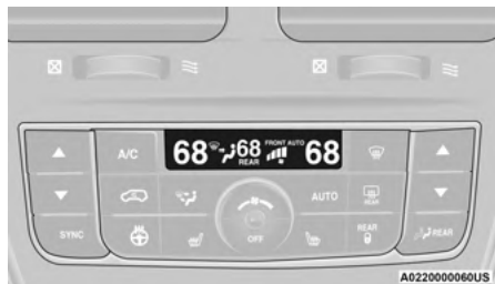
Automatic Temperature Controls
