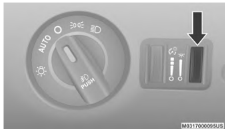
Ambient Light Dimmer Control
