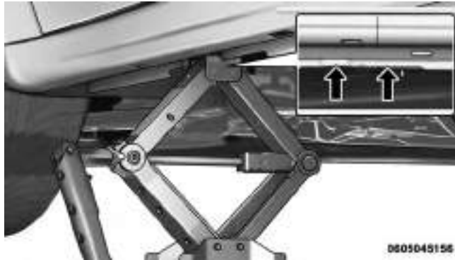
Front Jacking Location
