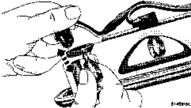
Pulling Bulb From Socket
