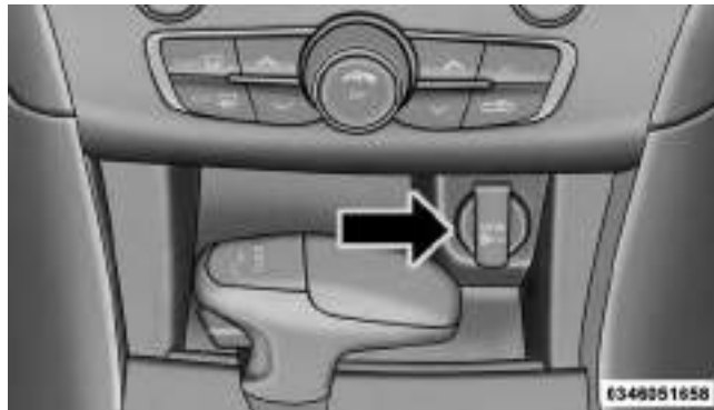
Front Power Outlet
