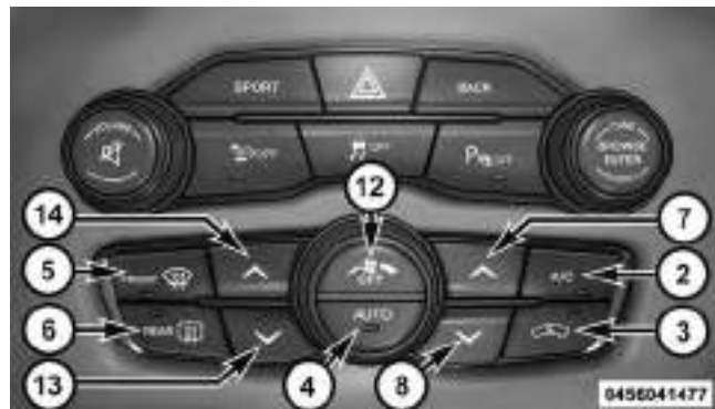
Automatic Climate Controls — Buttons On The Faceplate
