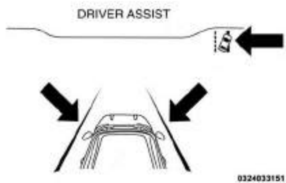
System ON (Gray Lines/White Indicator)
