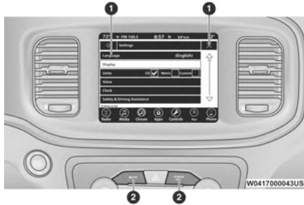
Uconnect 4C/4C NAV Buttons On The Faceplate And Buttons On The Touchscreen
