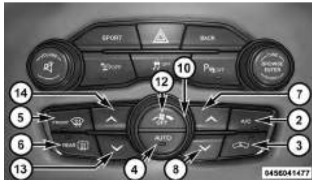
Automatic Climate Controls — Buttons On The Faceplate
