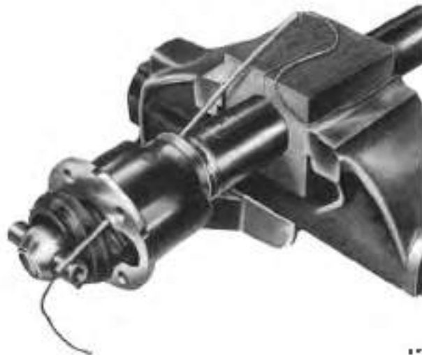
Fig. F8 Method of passing the cord through the tube (first position)
