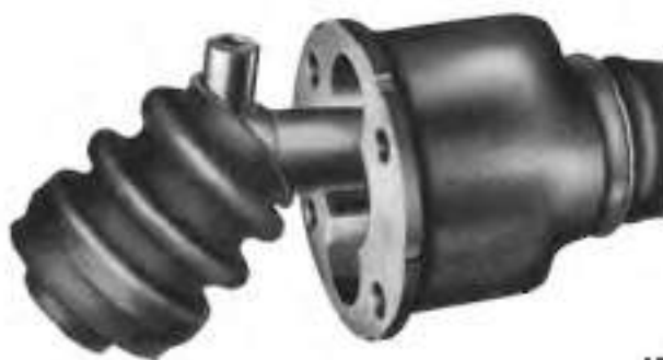
Fig. F7 Stretching the sealing boot over the trunnion pin
