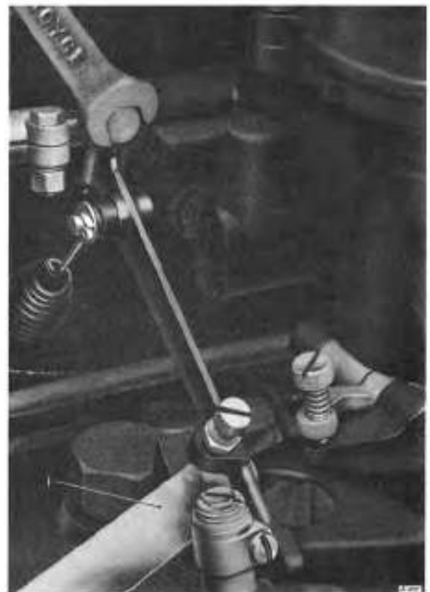
Fig. K14 Setting throttle lever — S1 cars
