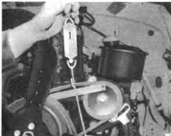
Fig. N6 Steering pump belt tension — to check
