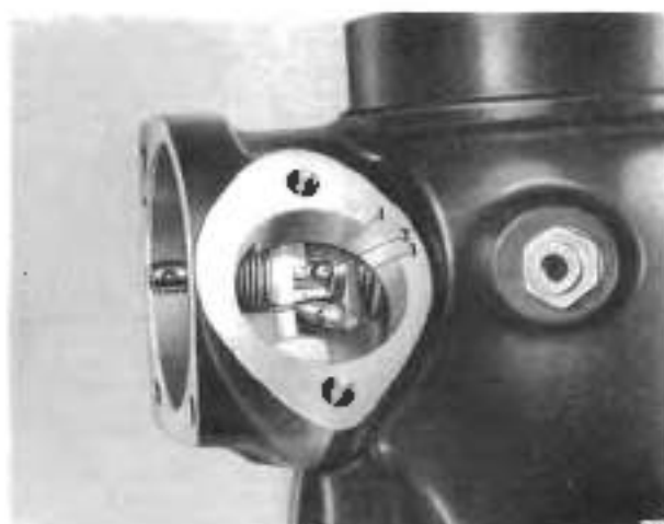
Fig. K19 Pick-up lever clearance — S2 cars
