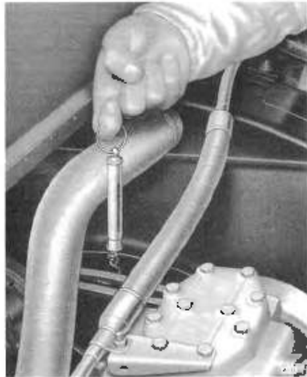
Fig. M3. Checking generator belt tension — S2 cars
