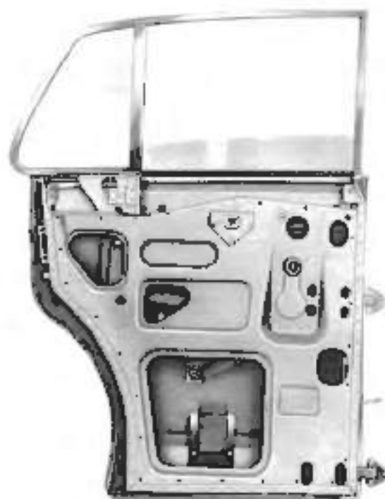
Fig. S17 Rear door with trim and finisher removed
