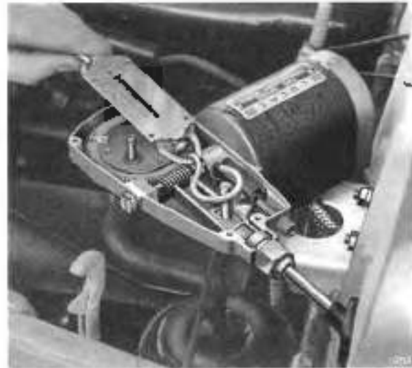
Fig. M50 Windscreen wiper load test
