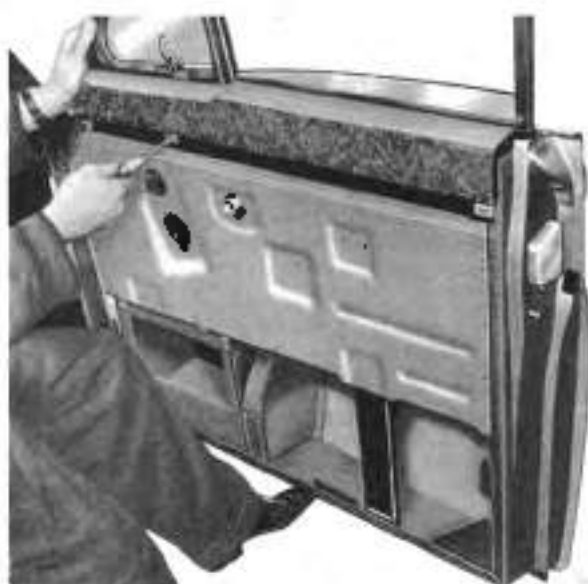
Fig. S2. Removing the finisher from the front door
