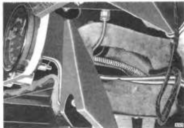
Fig. S42 Method of attaching anti-rattle felts to the instrument panel side plate and radio loudspeaker duct
