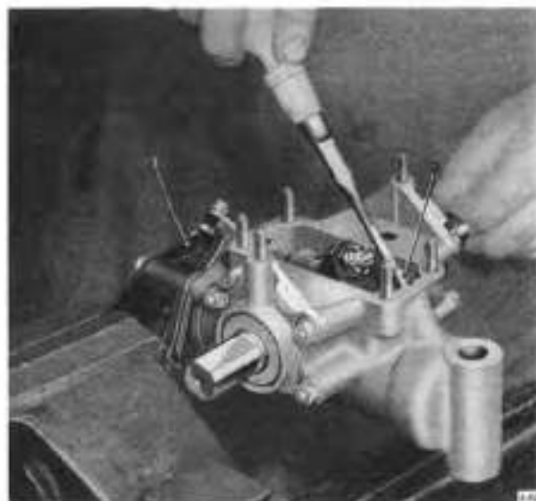
Fig. H26 Removing the bleed jets 1. MOUNTING PLATE HELD IN VICE 2. BLEED JET
