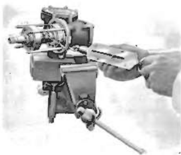
Fig. N27. Checking cross-load on spool valve
