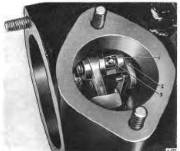
Fig. K18 Pick-up lever clearance — S1 cars
