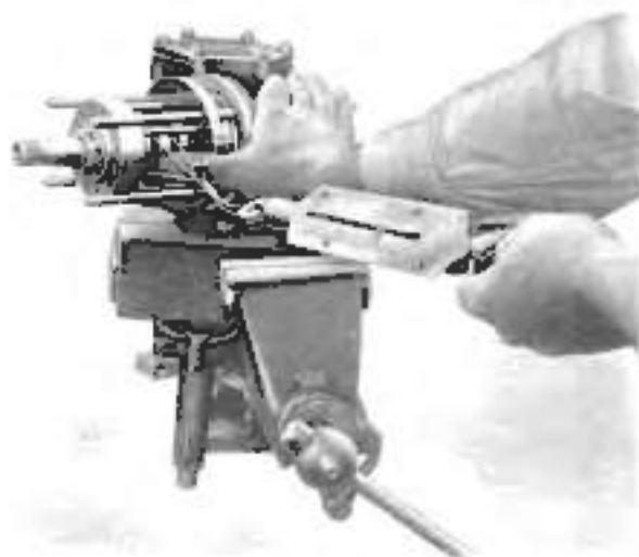
Fig. N28. Re-checking cross-load on spool valve
