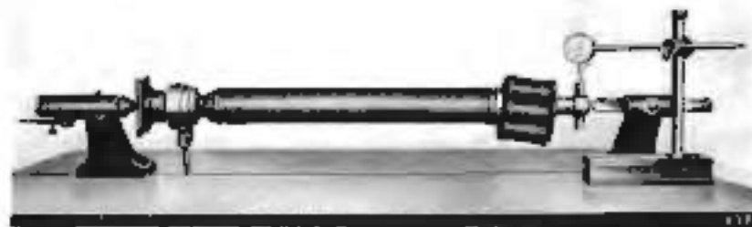
Fig. F6 Checking the centre pin
