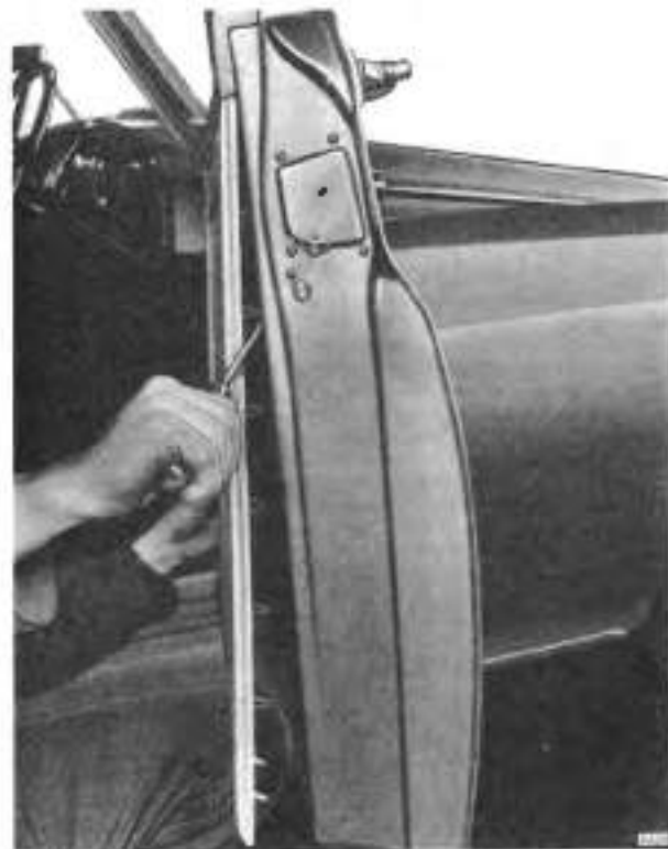
Fig. 51 Removing the trim from the front door
