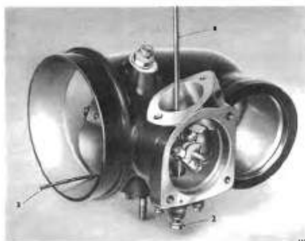
Fig. K20 Kick diaphragm adjustment — S2 cars
