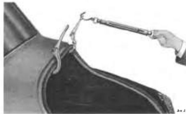
Fig. S36. Checking the luggage boot lid assistor weights.
