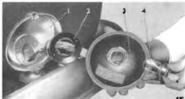
Fig. M45 Access to fog lamp bulb 1. LAMP BODY 3. LENS UNIT 2. CONTACT HOLDER 4. DOUBLE FILAMENT BULB
