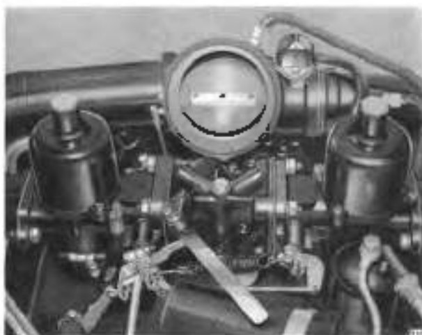
Fig. K15 Setting throttle lever — S2 cars
