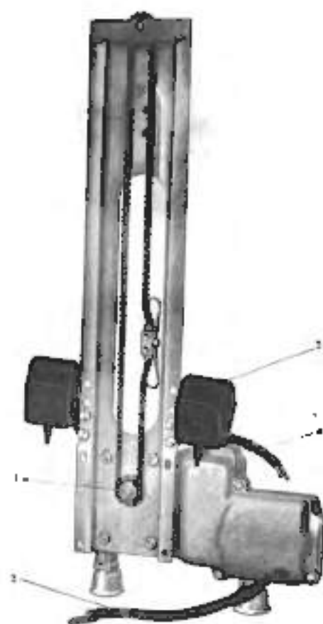
Fig. S19 Reverse side of motor and mechanism assembly for left-hand rear door
