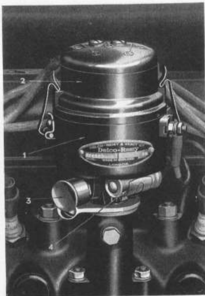
Fig. 39.—CONTACT BREAKER AND DISTRIBUTOR.
