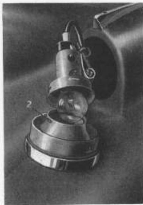
Fig. 49.—SIDE LAMP 2. Spring catch.
