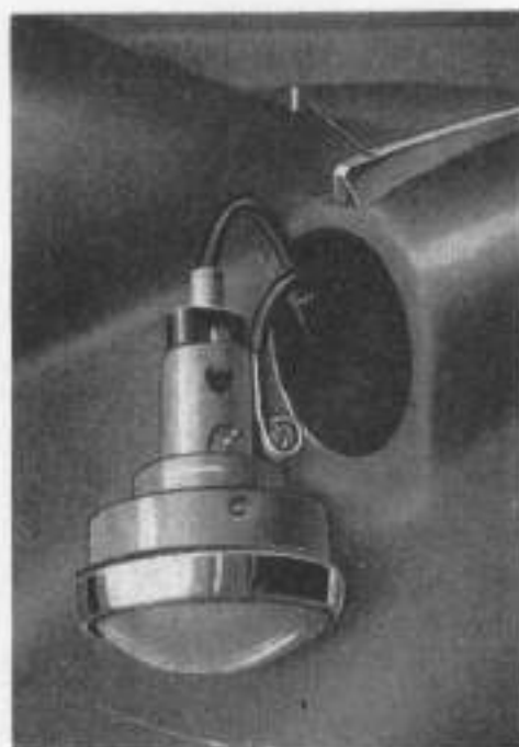
Fig. 48.—SIDE LAMP. 1. Locking screw.
