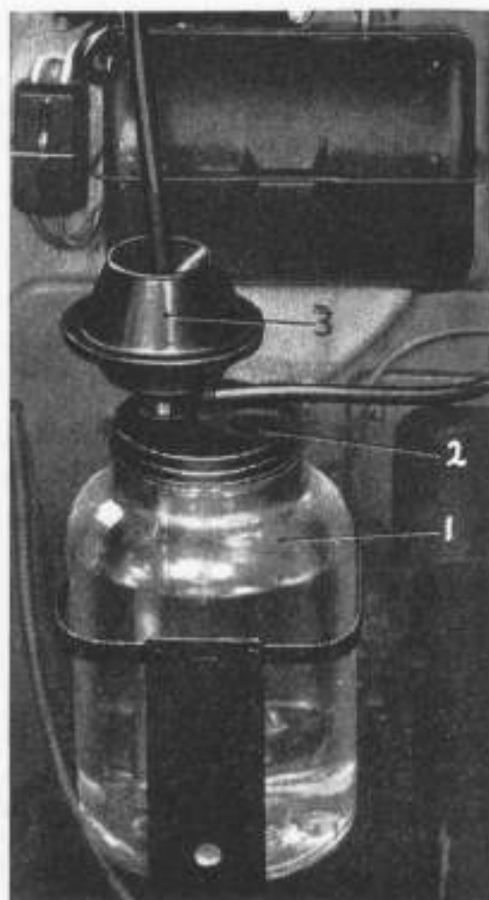
Fig. 52.—WINDSCREEN WASHER, RESERVOIR AND PUMP.
