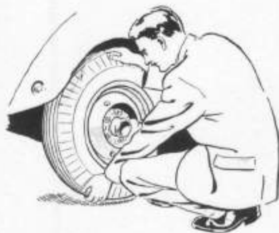
Fig. 28.—POSITIONING REAR WHEEL.
