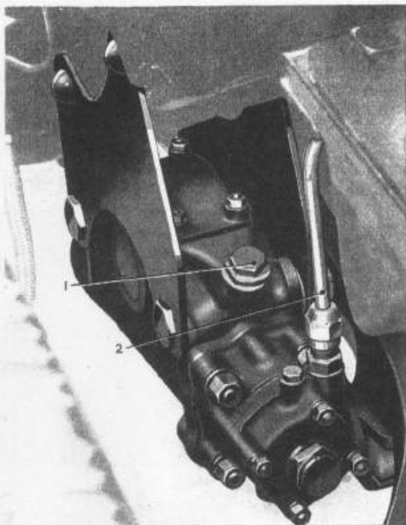
Fig. 24.—REAR HYDRAULIC SHOCK DAMPER.
