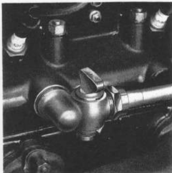
Fig. 35.—CAR HEATER CONNECTION AND ISOLATING TAP.
