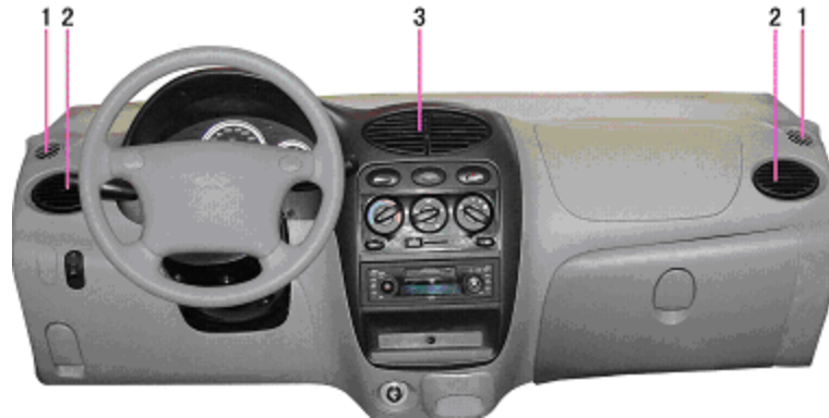
1、 Front windshield defroster ventilation opening 2、 Side ventilation opening 3、 Center ventilation opening
