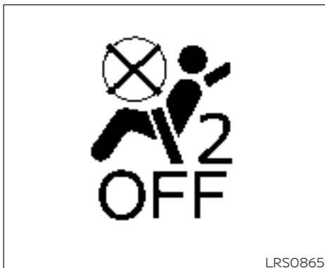
Front passenger air bag and status light
