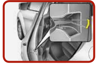
Emergency door locking [4]
