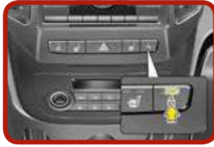
Operating door locks from inside the vehicle with central door lock switch [4]
