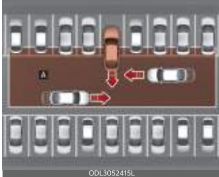
[A]: Rear Cross-Traffic Collision Warning operating range
