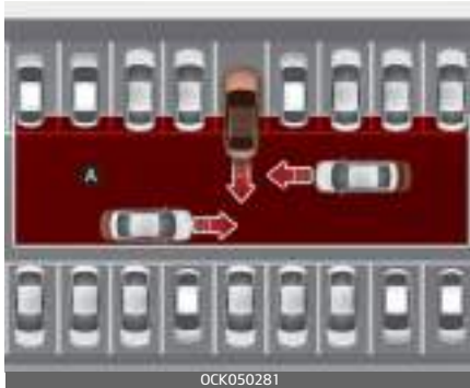
[A]: Rear Cross-Traffic Collision Warning operating range
