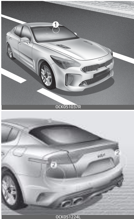
[1] : Front view camera, [2] : Rear corner radar
