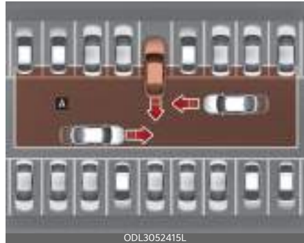
[A]: Rear Cross-Traffic Collision Warning operating range
