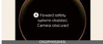
A: Forward safety systems disabled. Camera obscured
