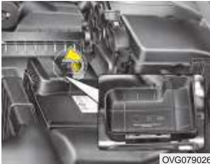
Engine room (Battery terminal cover)
