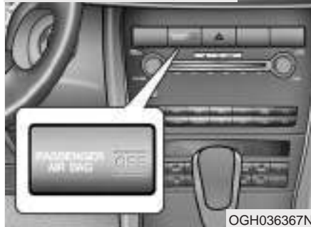
The location of OCS warning indicator
