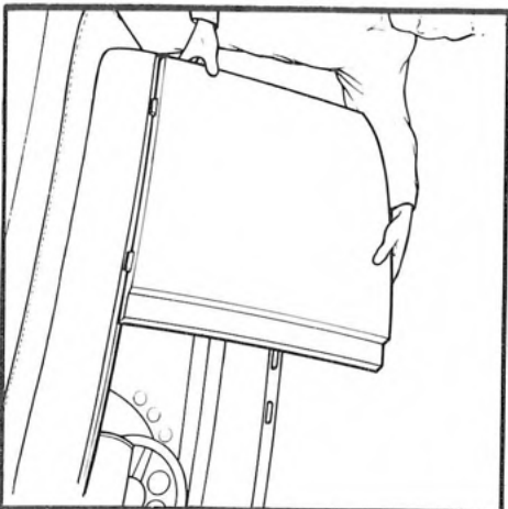
Fig. 22 Erecting Passenger Roof Panel.
