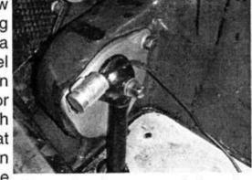
Above: Condenser mounted on the cover plate.
