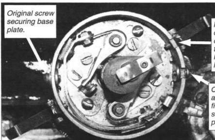
New slot 30 degrees from original to locate the modern cap. Fit new screws to hold spring clips.
