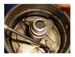
Automatic advance and retard weights and springs. Check for breakage or seizure
