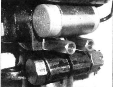
Above: Photographs above showing the two M4 securing screws replaced by two studs loctited to the body of the distributor on which you can 'hook' the spare condenser.
