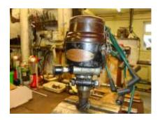
The distributor showing cap and leads. Condenser is under distributor body. Greaser on the left
