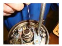
Setting the gap to 18 thou using adjustment screw
