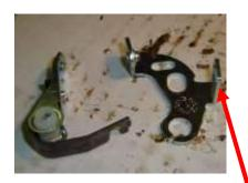
A new set of points. It is necessary to saw off the square lug on the fixed contact
