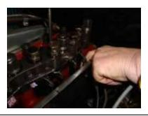
Checking TDC at the valves. Inlet and exhaust pushrods rotate
