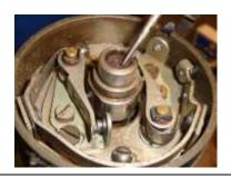
Rotor arm removed showing felt pad. Oil sparingly from time to time
