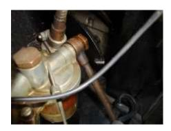
Strobe lead attached to plug lead 1
