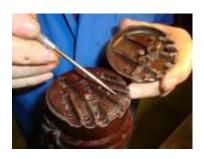
Exterior of Delco cap showing impaling spikes. Seal cable exits with silicone to prevent water ingress
