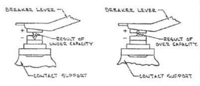
Fig. 13.--PITTED CONTACT POINTS CAUSED BY USING CON-DENSER WITH INCORRECT CAPACITY
