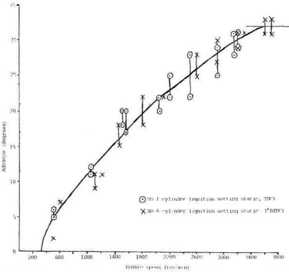
Timing measurements with Delco-Remy unit (650 KB). Vertical lines represent ignition scatter. Governor range 33° approximately (at crankshaft). Cut-off speed 1800 rev/min (3600 rev/min at crankshaft). Static ignition settings measured using small lamp across points.
