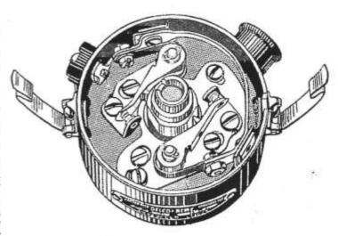
Above: The dual contact breakers fitted to 6 cylinder Talbot cars.
