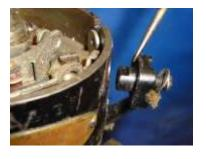
Remove base plate by removing two spring clip screws
