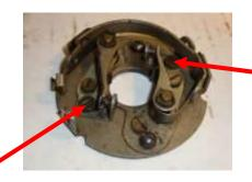
Base plate. Remove points by undoing marked screws (red arrows). The upper and lower screws on the right hold the base plate and should not be touched
