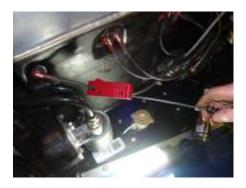
Transposed timing mark. Easier to line up on chassis member
