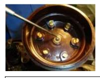
Interior of Delco cap. Check carbon button and brass contacts
