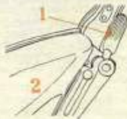
1. Lower tail gate handle 2. Lower tail gate
