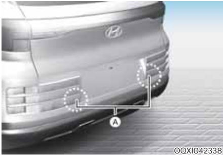
[A] : Rear ultrasonic sensors
