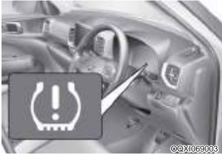
Low tire pressure telltale / TPMS malfunction indicator
