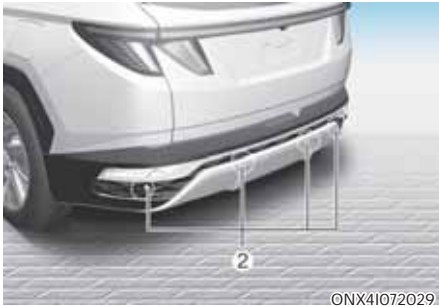
[2] : Rear ultrasonic sensors
