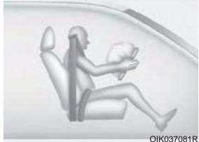
When the SRSCM detects a sufficiently severe impact to the front of the vehicle, it will automatically
