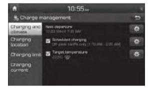
You can set the date and time of when to charge the battery and the climate control temperature. Also, you may select the time to start charging using the off-peak time setting.
