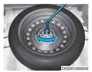
If it is hard to loosen the tire holddown wing bolt by hand, you can loosen it easily using the wheel nut wrench.
