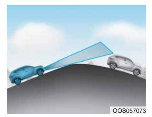
When coasting on an uphill or downhill, the system may not detect the vehicle in your lane and the regenerative braking level will reduce automatically, making you feel that the vehicle is accelerating.
