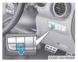
You may select when the charging connector can be locked and unlocked in the charging inlet. Press the setup between AUTO mode and LOCK mode.
