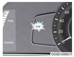
This warning light illuminates if the START/STOP button is changed to the ON position and goes off in approximately 3 seconds if the system is operating normally.
