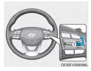
(RES+) and hold it, while monitoring the set speed on the instrument cluster.
