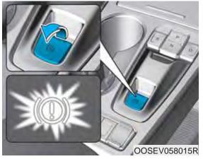
To apply the EPB (Electronic Parking Brake):
