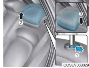
Removal/Reinstallation To remove the headrest:
