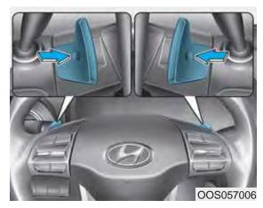
The paddle shifter is used to adjust the regenerative braking level from 0 to 3 during decelerating or braking.
