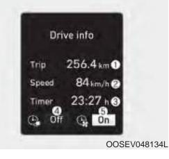
At the end of each driving cycle, the Driving Info message is displayed. This display shows the trip distance (1), average vehicle speed (2), driving time (3), charging time status (4) and climate time status (5).
