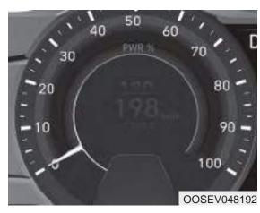
The torque gauge shows the realtime torque value while driving when SPORT mode is selected by pressing the DRIVE MODE button. Power/Charge gauge
