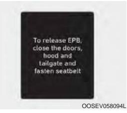
To release EPB, close the doors, hood and tailgate and fasten seatbelt
