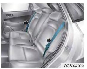
3.Locate the seatbelt toward the outboard position before folding down the seatback. If not, the seatbelt system may be interfered by the seatback.
