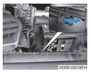
If the charging connector does not disconnect due to battery discharge and failure of the electric wires, open the hood and slightly pull the emergency cable. The charging connector will then disconnect.
