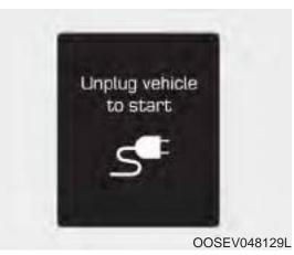
This message is displayed when you start the vehicle without unplugging the charging cable. Unplug the charging cable, and then turn on the vehicle. Charging door open
