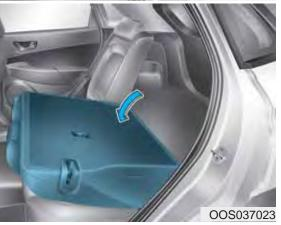
4.Remove the belt from the guide (1) and pull up the seatback folding lever (2), then fold the seat toward the front of the vehicle.
