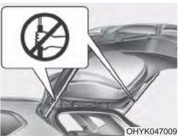
Do not hold the part (gas lifter) that supports the tailgate. Be aware that the deformation of the part may cause vehicle damage and a risk of safety accident.
