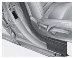
All specifications (sizes and pressures) can be found on a label attached to the driver's side center pillar.
