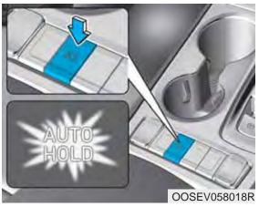
1. With the driver's door, hood and tailgate closed, depress the brake pedal and then press the [AUTO HOLD] switch. The white AUTO HOLD indicator will come on and the system will be in the standby position.
