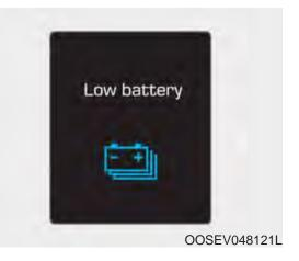
When the high voltage battery level reaches below approximately 8%, this warning message is displayed.
