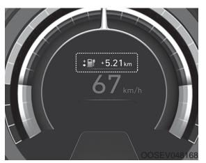
The additional distance to empty which is converted from the energy regenerated by the regenerative braking is displayed if the ECO/ECO+ mode is selected by pressing the Drive Mode button. The display is initialized to 0 if the regenerative braking stops because of acceleration, etc. Reduction gear shift indicator
