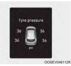
• You can check the tire pressure in the Assist mode on the cluster.
