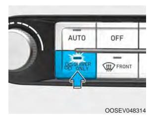
If you press the DRIVER ONLY button(\* DRIVER) and the indicator light illuminates, cold air mostly blows in the direction of the driver's seat. However, some of the cold air may come out of other seating position ducts to keep indoor air pleasant.
