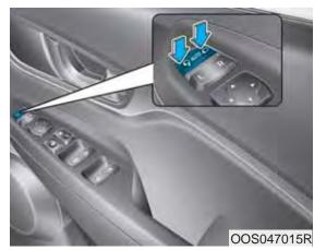
Electric type (if equipped) Left : The mirror will unfold. Right : The mirror will fold.
