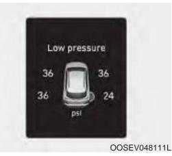
This warning message is displayed if the tire pressure is low. The corresponding tire on the vehicle will be illuminated.
