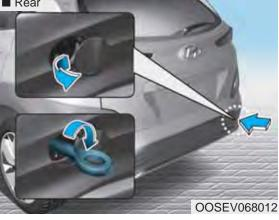
2. Remove the hole cover by pressing the lower part of the cover on the bumper.
