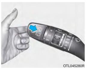
In the OFF position, pull the lever gently toward you to spray washer fluid on the windshield and to run the wipers 1-3 cycles. The spray and wiper operation will continue until you release the lever. If the washer does not work, you may need to add washer fluid to the washer fluid reservoir.
