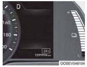
This gauge indicates the current outside air temperatures either in Celsius (°C) or Fahrenheit.
