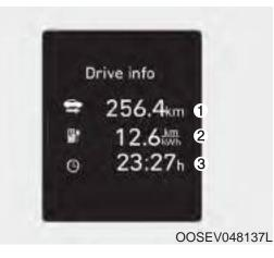
This display shows the trip distance (1), the average energy consumption (2), and the total driving time (3).
