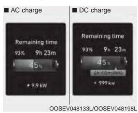
This message is displayed to notify the remaining time to charge the battery to the selected target battery charge level. Unplug vehicle to start
