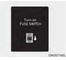
If the fuse switch is OFF, "Turn on FUSE SWITCH" message will appear.
