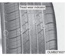
If the tire is worn evenly, a tread wear indicator will appear as a solid band across the tread. This shows there is less than 1.6 mm (1/16 in.) of tread left on the tire. Replace the tire when this happens.
