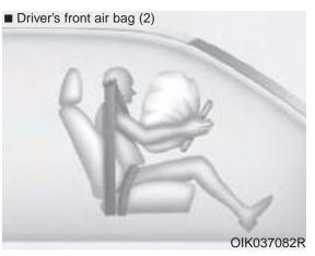
Upon deployment, tear seams molded directly into the pad covers will separate under pressure from the expansion of the air bags. Further opening of the covers allows full inflation of the air bags.
