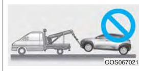
Do not tow with sling-type equipment. Use wheel lift or flatbed equipment.
