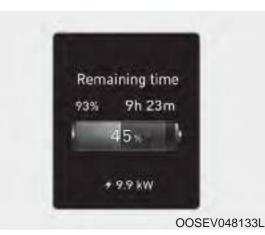
9. After charging has started, the estimated charging time is displayed on the instrument cluster for about 1 minute.
