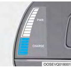
The Power/Charge gauge shows the energy consumption rate of the vehicle and the charge/discharge status of the regenerative brakes.
