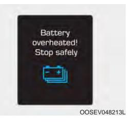
This warning message is displayed to protect battery and electric vehicle system when the high voltage battery temperature is too high.
