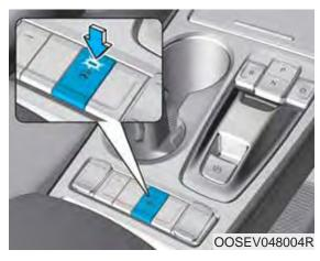
When the vehicle is ON, press the heated steering wheel button to warm the steering wheel. The indicator on the button will illuminate.
