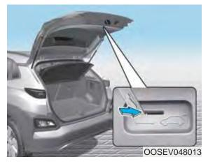
emergency tailgate safety release lever located on the bottom of the tailgate. When someone is inadvertently locked in the luggage compartment. The tailgate can be opened by doing as follows:
