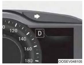
The indicator in the instrument cluster displays the gear position when the START/STOP button is in the ON position.
