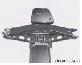
Mount the jack after being fastened the spare tire to the bar when you install the jack.
