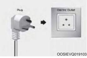
4.Disconnect the plug from the household electric outlet. Do not pull the cable when disconnecting the plug.
