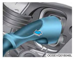
1.Hold the charging connector handle and pull it out.
