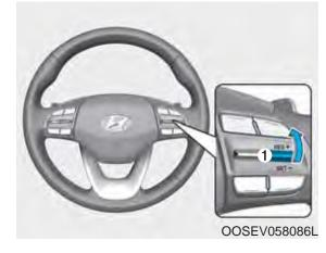
(RES+). If the vehicle speed is over 30 km/h (20 mph), the vehicle will resume the preset speed.
