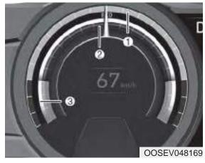
The Smart Eco Pedal Guide is displayed to lead to eco-driving when you press the DRIVE MODE button and select ECO/ECO+ mode.
