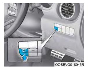
The Virtual Engine Sound System generates engine sound for pedestrians to hear vehicle sound because there is no sound while the Electric Vehicle (EV) is operating.
