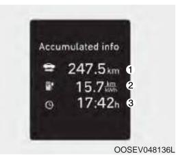
This display shows the accumulated trip distance (1), the average energy consumption (2), and the total driving time (3).
