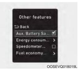
The driver can activate the Aux. Battery Saver+ function by placing the START/STOP button to the ON position and by selecting:
