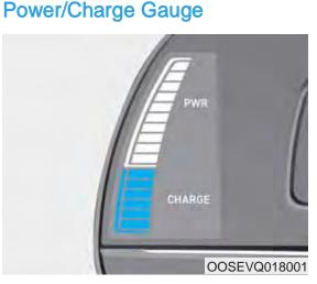
The Power/Charge Gauge shows the energy consumption rate of the vehicle and the charge/discharge status of the regenerative brakes.
