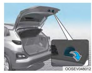
Lower the tailgate lid and press down until it locks. To be sure the tailgate lid is securely fastened, always check by trying to pull it up again.
