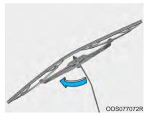
1. Raise the wiper arm and turn the wiper blade assembly to expose the plastic locking clip.
