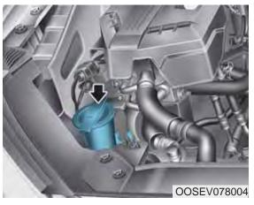
fluid reservoir and add fluid if necessary. Plain water may be used if washer fluid is not available. However, use washer solvent with antifreeze characteristics in cold climates to prevent freezing.
