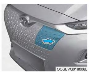
3. Push the charging door where the icon is located to open. The charg-ing door opens only when the door is unlocked.
