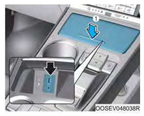
You can use an AUX port to connect audio devices and an USB port to plug in an USB and an iPod® port. To use the AUX, USB and iPod®, open the front console cover by slightly pressing the lower part of the cover (1).
