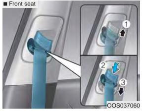
To adjust the height of the seat belt anchor, lower or raise the height adjuster into an appropriate position. To raise the height adjuster, pull it up (1). To lower it, push it down (3) while pressing the height adjuster button (2).
