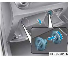
1. With the glove box open, remove the stoppers on both sides.
