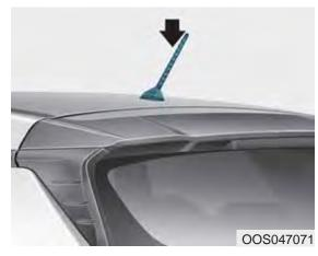
The roof antenna receives transmitted data. (For example : AM/FM)
