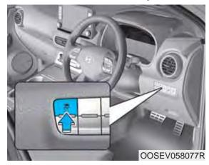
(ESC) system helps to stabilize the vehicle during cornering maneuvers.
