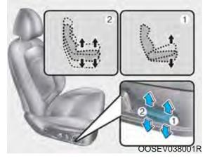
Seat cushion tilt (1, if equipped) To change the angle of the front part of the cushion:
