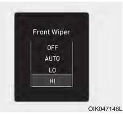
This indicator displays which wiper speed is selected using the wiper control.
