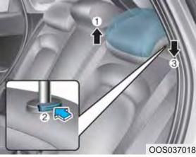
Adjusting the height up and down To raise the headrest:
