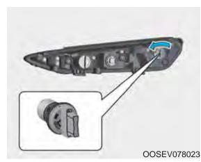
5. Insert a new bulb by inserting it into the socket and rotating it until it locks into place.
