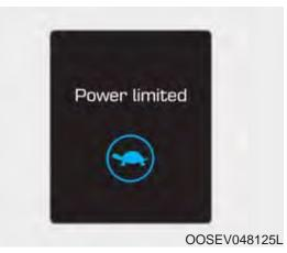
In the following cases, this warning message is displayed when the vehicle's power is limited for safety.
