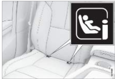
Mounting point locations for the front seat are indicated by symbols on the upholstery of the backrest.
