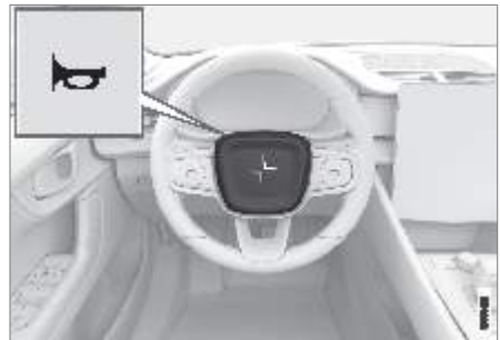
The horn is located in the centre of the steering wheel.
