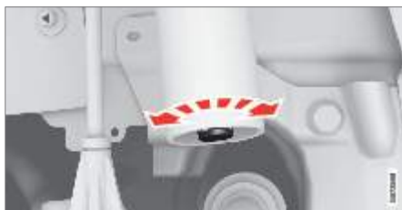
Turn the adjusting knob clockwise or counterclockwise to change the adjustment position.
