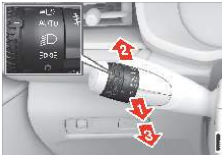
Steering wheel stalk switch with rotating ring.
