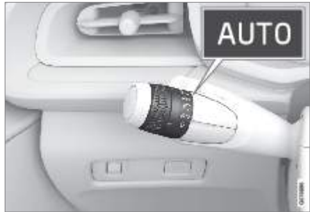
Stalk switch rotating ring in AUTO position.
