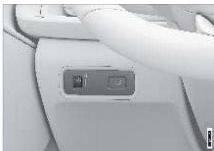
Thumbwheel (to left) for adjusting interior brightness.
