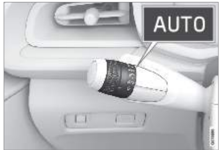
Stalk switch rotating ring in AUTO position.
