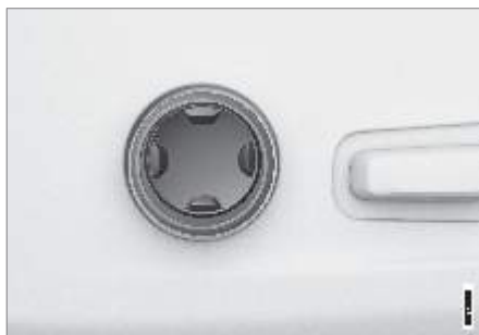
Four-way button that controls the car's four-way lumbar support.
