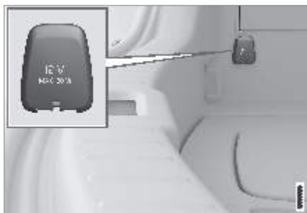
12 V electrical socket in cargo area.
