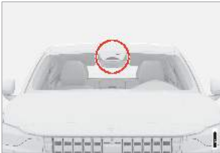
Location of the camera unit
