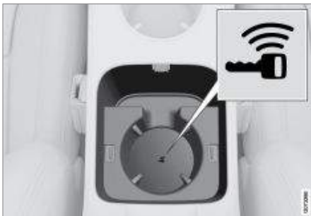
Backup reader's location in the tunnel console.
