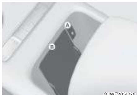
[A] : Indicator light, [B] : Charging pad
