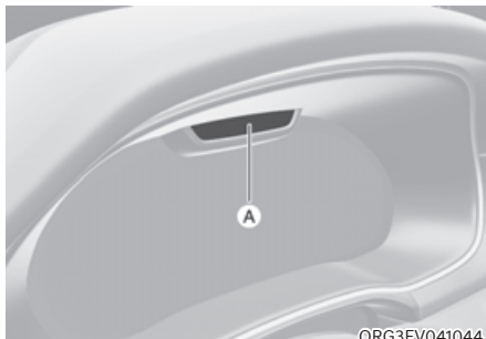
[A] : Interior view camera
