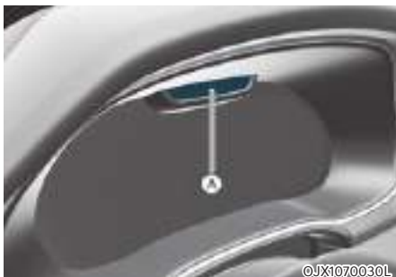
[A] : Interior view camera
