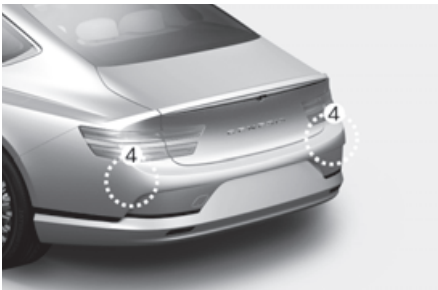
[1]: Front view camera, [2]: Front radar, [3]: Front corner radar (if equipped), [4]: Rear corner radar
