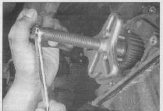
7.2 Attach a bolt-type gear puller to the crankshaft sprocket and remove the sprocket from the crankshaft
