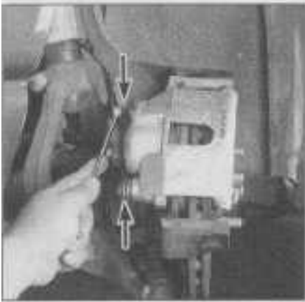
3.4a To remove the front brake caliper, remove the two guide pin bolts (arrows)
