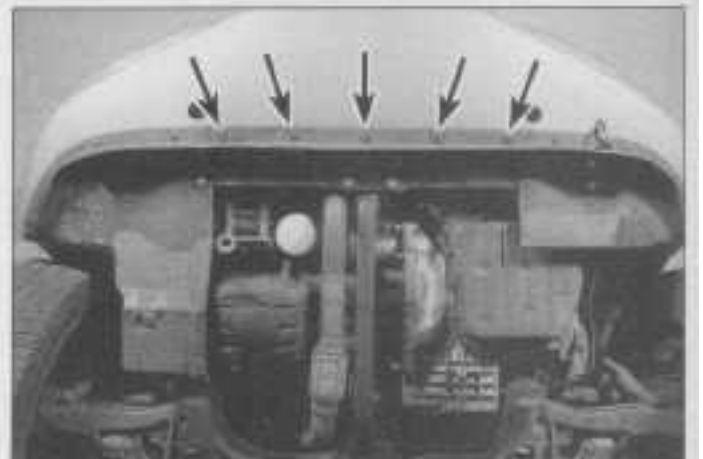
12.5 Remove the five push-in fasteners (arrows) securing the bottom of the front bumper to the radiator lower support
