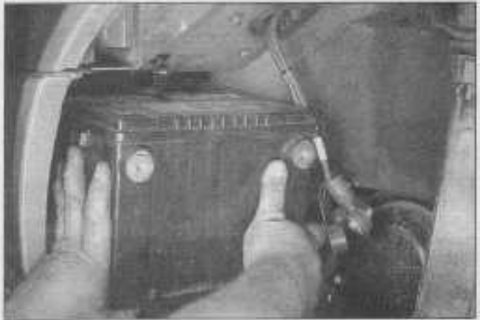
4.7 Position the cables out of the way and slide the battery out of the fenderwell - be careful, it's heavy!
