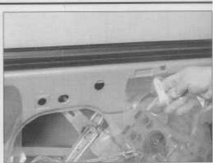
15.2 Remove the plastic water shield from the door
