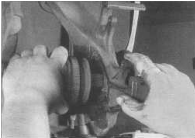
8.8a Angle the steering knuckle as required and pull the driveaxle from the wheel hub
