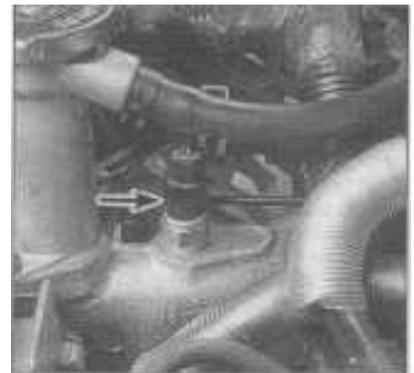
4.3 The coolant temperature sensor (arrow) is located at the front of the engine, next to the thermostat
