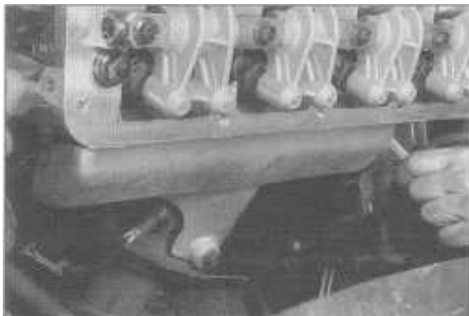
5.5 Remove the exhaust manifold heat shield mounting bolts (arrows) and remove the heat shield
