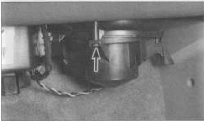
9.11 Remove the screws retaining the blower motor to the heater housing (arrow)
