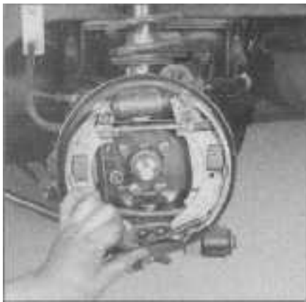
6.4b Remove the lower return spring - note that the shorter spring end is towards the trailing brake shoe
