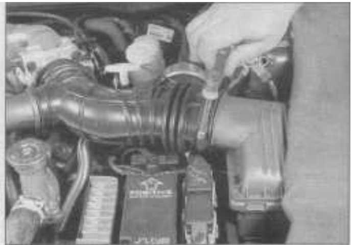
9.4a Loosening the air duct clamp at the air filter housing (V6 engine shown, others similar)
