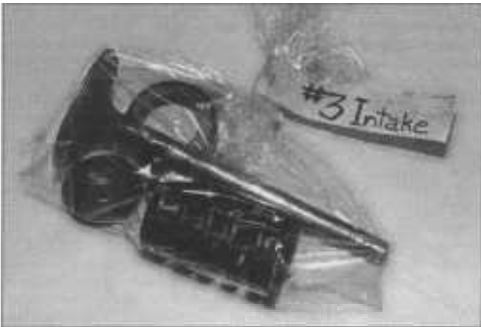
10.2 A small plastic bag with an appropriate label can be used to store the valvetrain components so they don't get mixed up
