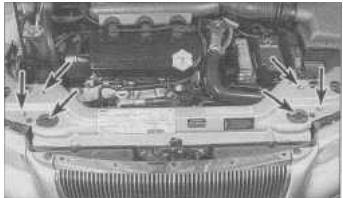
4.7 Remove the four bolts and the isolators on the upper radiator crossmember (arrows) - if necessary, remove the bolts securing the shroud and remove the shroud
