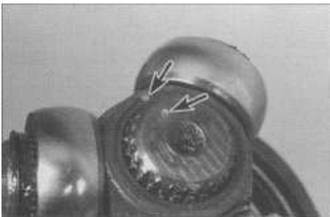
9.25 Use a centerpunch to mark (arrows) the tripod spider to the axle shaft
