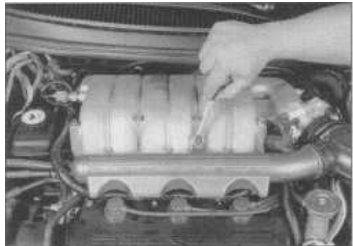
9.1b Removing the air inlet resonator bolt (V6 engine)
