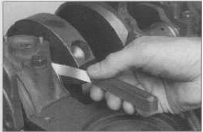
16.3 Checking the crankshaft endplay using feeler gauges at the thrust bearing journal
