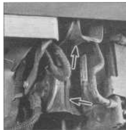
21.12 The horns (arrows) are located behind the front bumper on the right side frame rail, one above the other
