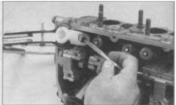
10.3 After compressing the valve spring, use a magnet (shown) or needle-nose pliers to extract the valve keepers - a valve spring compressor adapter, such as the one shown, will be needed to compress the valve spring on this type of cylinder head
