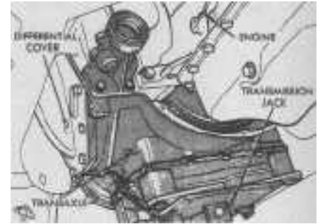
9.34 Using a transmission jack to remove the transaxle
