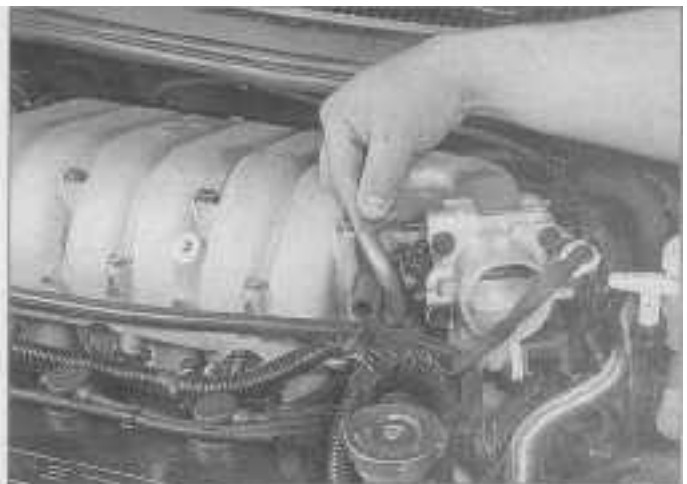
4.3b Disconnect the purge vacuum hose from the throttle body fitting
