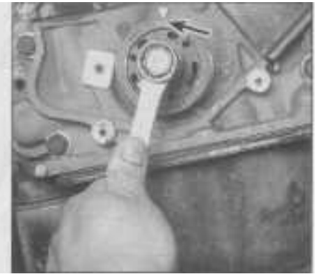
6.21a On 2.0L engines, use a box-end wrench or socket to rotate the crankshaft timing sprocket until the TDC mark on the sprocket is aligned with the arrow on the oil pump housing (arrow) . . .
