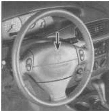
29.1a The driver's side airbag (arrow) is located in the steering column horn pad
