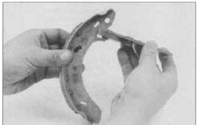
6.4p Install the automatic self-adjuster onto the proper leading brake shoe (they are unique for each side of the vehicle, RH or LH and are marked on the reinforcement plate) - after installation the quadrant teeth should be on the reinforced side of the brake shoe
