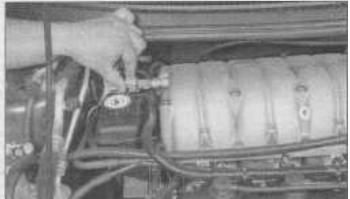
3.41 Disconnecting the electrical connector from the IAT sensor - V6 engine shown
