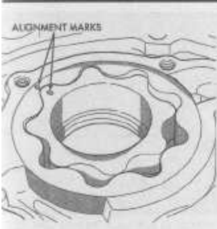
14.16a Install the rotors into the oil pump body with the match marks aligned
