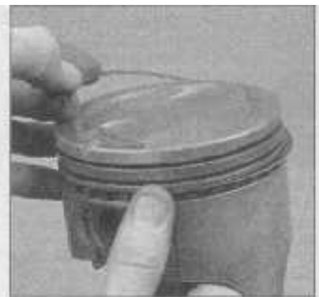
24.9b DO NOT use a piston ring installation tool when installing the oil control side rails
