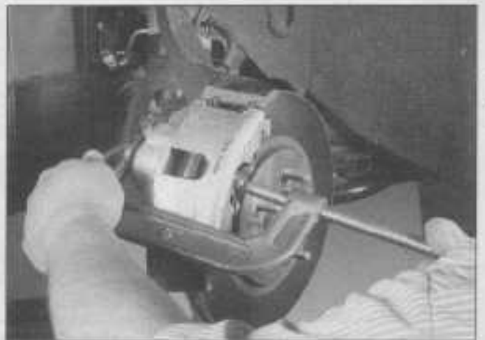
3.3 Use a C-clamp to press the caliper piston into its bore
