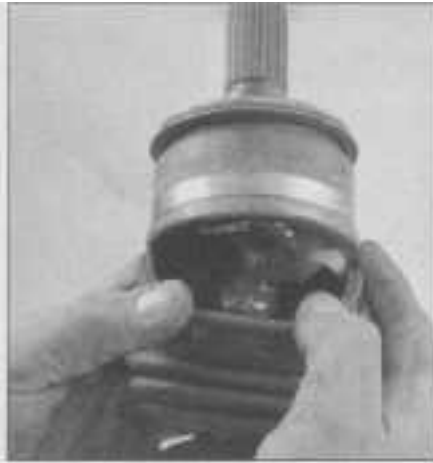
9.4 Remove the boot from the CV joint housing
