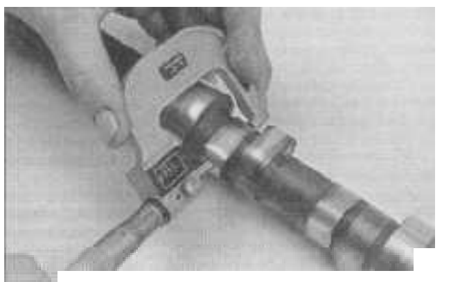
10.10 Check the camshaft lobes for wear with a micrometer
