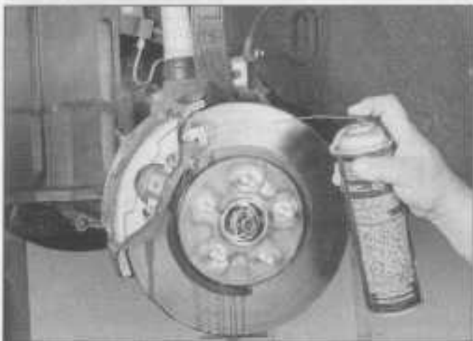
3.2 Always wash the brakes with brake system cleaner before working on them
