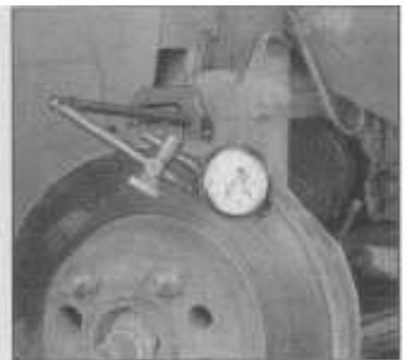
5.3 Use a dial indicator to check disc runout - if the reading exceeds the specified runout limit, the disc will have to be machined or replaced
