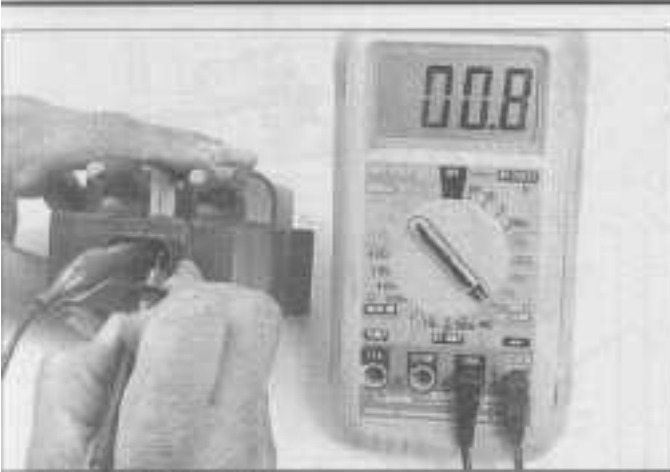
7.4 Test each coil's primary resistance by connecting one probe of the ohmmeter to the center terminal and the other probe to each end terminal. The primary resistance of each coil should be within specifications
