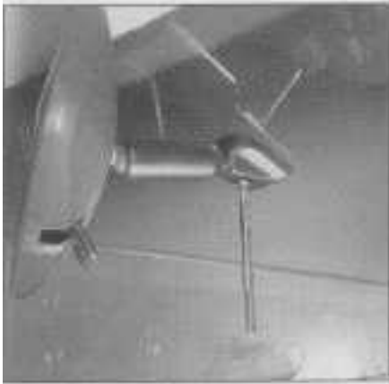
27.1a The interior mirror mounts to a button which is bonded to the windshield and is held in place by a set screw - loosen this screw . . .
