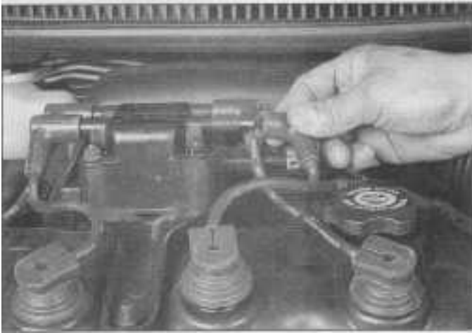
27.7a Pull on the spark plug wire boot and twist it back-and-forth while pulling it from the ignition coil pack
