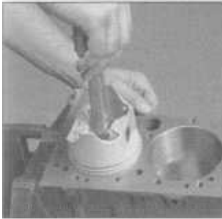
24.3 Install the piston ring into the cylinder then push it down into position using a piston so the ring will be square in the cylinder
