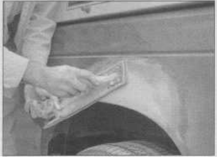
8 Use coarse-grit sandpaper and a sanding board or block to work the filler down until it's smooth and even. Work down to finer grits of sandpaper - always using a board or block - ending up with 360 or 400 grit
