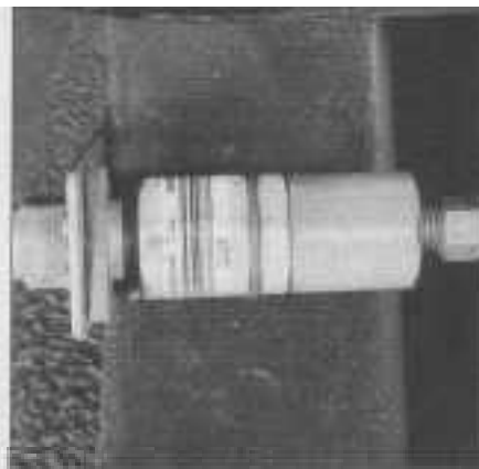
9.10 On 1998 and later models equipped with ABS, the proportioning valves are located in the rear wheel well and mounted on the upper frame rail between the metal brake line and the brake hose
