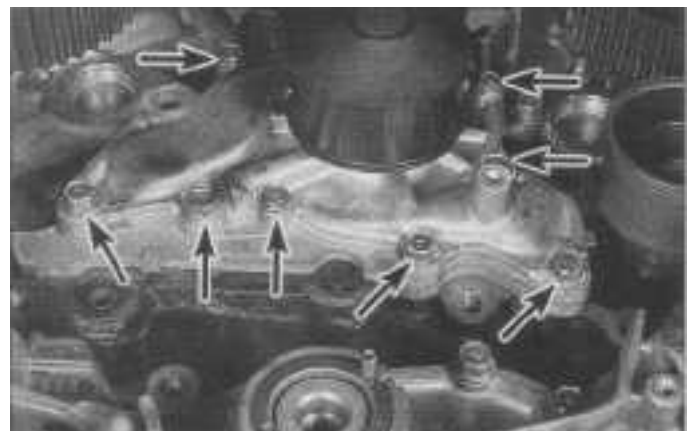
7.18 Remove the water pump bolts (arrows) - V6 engine
