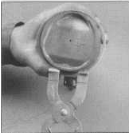
20.2 Use a piston ring removal tool (shown) to remove the rings from the pistons
