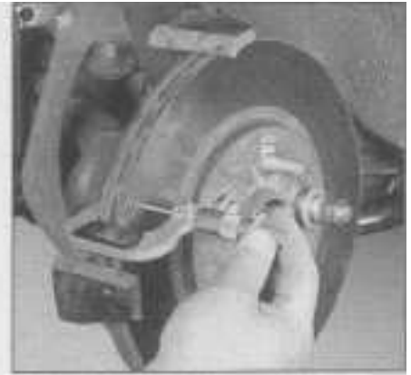
5.4b Use a micrometer to measure the thickness of the disc at several locations
