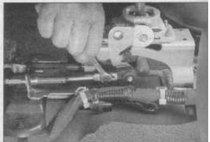
2.18 Loosen the crossover cable adjusting bolt
