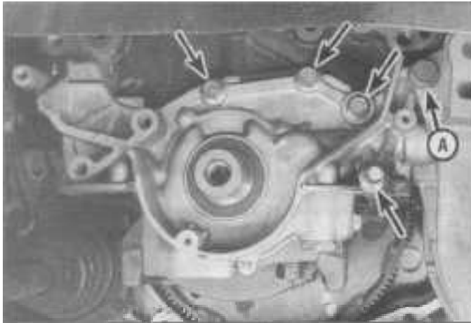
14.7 Remove the oil pump assembly mounting bolts (arrows) and detach it from the engine - bolt (A) also secures the air conditioning compressor bracket (if equipped)
