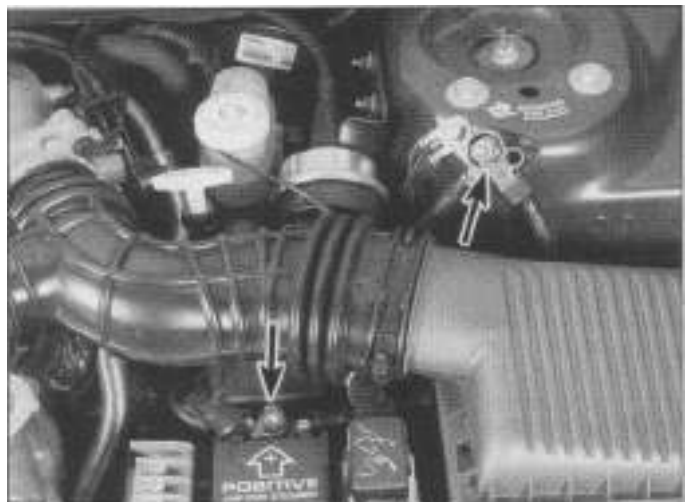
The remote battery terminals (arrows) are located in the engine compartment and well marked - when connecting jumper cables connect the cable to the positive terminal first, then the negative terminal
