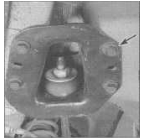
12.3 Unbolt the trailing link bracket bolts (arrow) to remove the forward end of the trailing link
