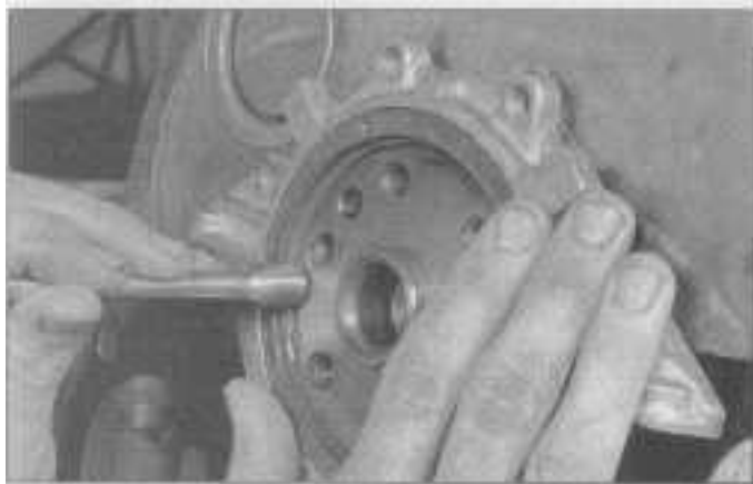
16.12 Using a rounded object like a socket extension, carefully work the seal onto the crankshaft
