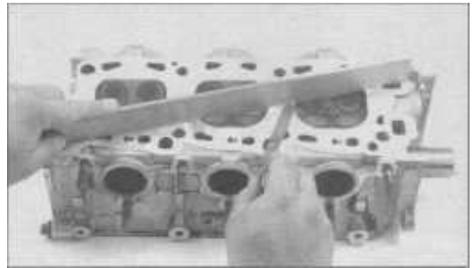
12.19a Checking the cylinder head-to-engine block gasket surface for warpage
