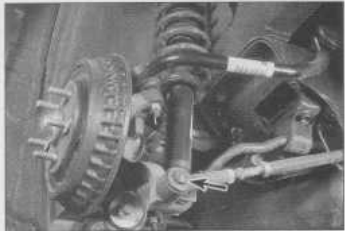
13.6 Remove the rear lateral link to knuckle bolt (arrow) and nut
