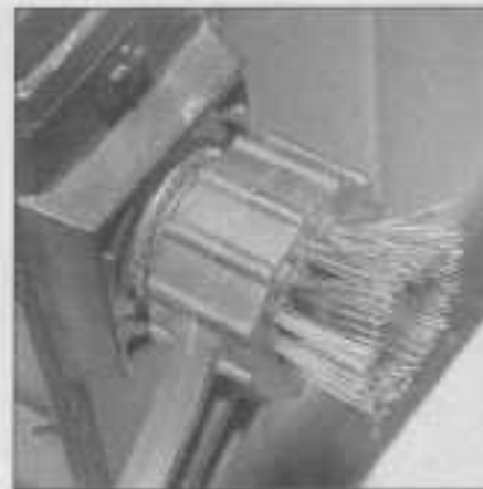
9.6b The side terminal battery brush includes a special ring-type portion used to clean the battery cable sealing recess around the terminal
