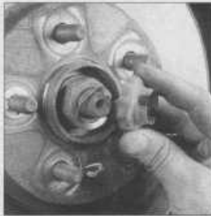
8.2b ... then remove the lock and spring washer
