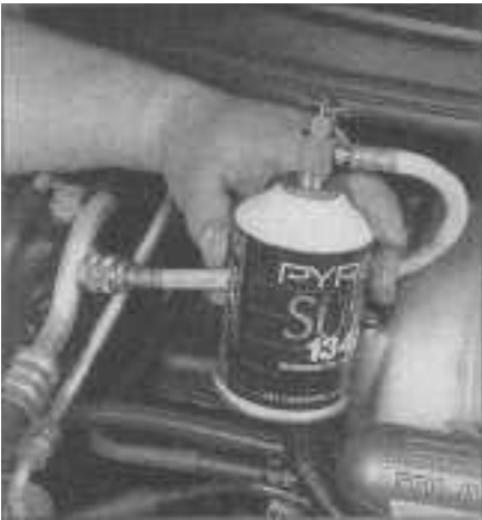
12.12 Cans of R-134A refrigerant are available in auto parts stores that can be added to your system with a simple recharging kit
