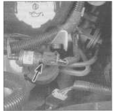
6.10 EGR solenoid/transducer (arrow) - V6 engine shown
