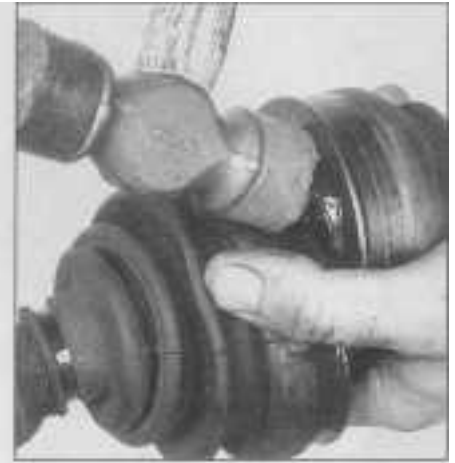
9.5a Use a soft-faced hammer to disengage the outer CV joint from the axle shaft retaining circlip ..
