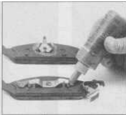
3.4h Apply an anti-squeal compound to the backs of the pads where they mate with the caliper and piston
