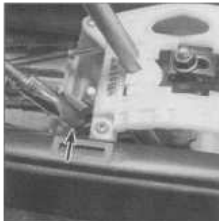
7.21 Loosening the interlock cable adjusting nut (arrow)
