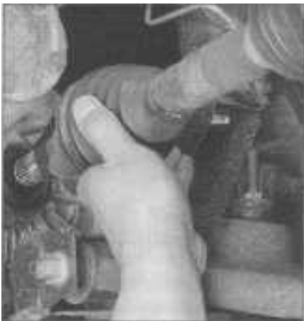
8.11 To avoid damaging the transaxle oil seal, support the ends of the driveaxle and pull it straight out
