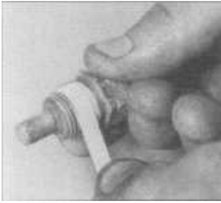
3.37 If you're re-installing the old ECT sensor, wrap the threads with Teflon tape to prevent leakage
