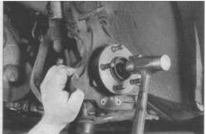
8.8b If the driveaxle is stuck in the wheel hub, apply some penetrating oil to the hub splines then install the hub nut onto the driveaxle a few turns (to protect the threads) and strike the end of the driveaxle with a soft-faced hammer to break it loose - DO NOT attempt to drive the driveaxle out of the hub using a hammer!
