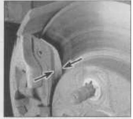
18.5 Measure the thickness of the brake pad from the metal backing to the brake disc - note the inner pad generally wears faster than the outer pad so measure both of them
