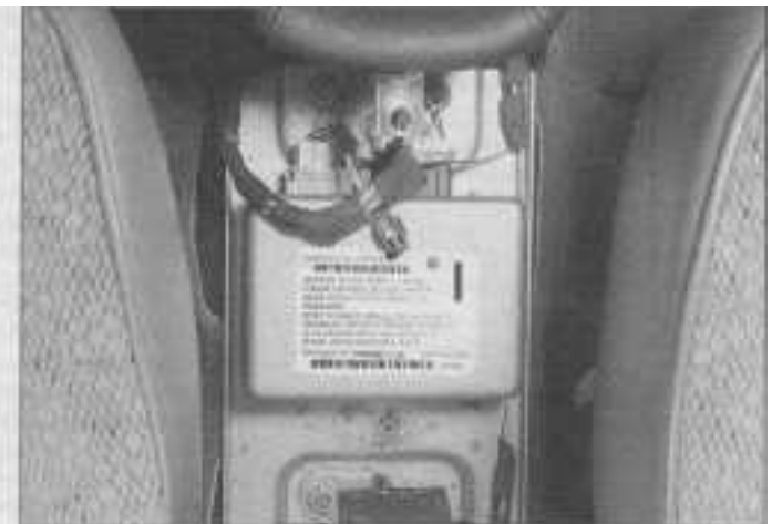
29.1c The Airbag Control Module is located under the center console and mounted to the floorpan
