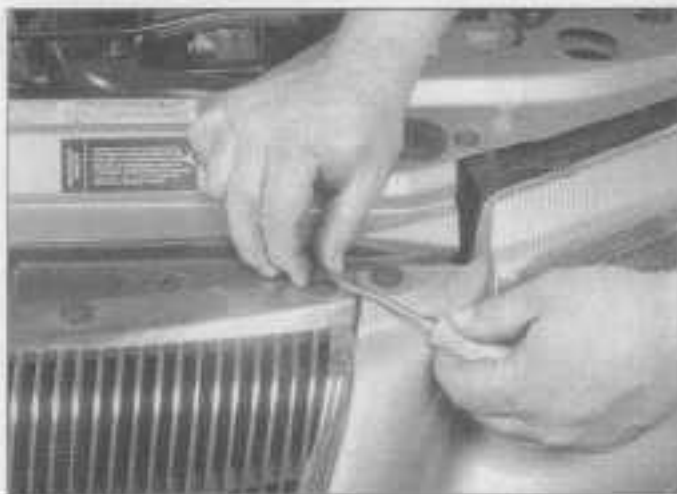
12.7 To remove the push-in fasteners, pry out the center stud and then remove the outer housing
