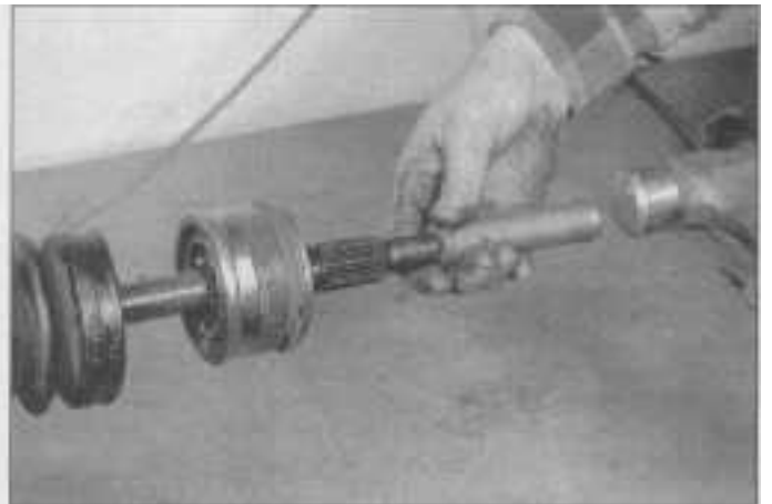
9.12 Install the outer CV joint onto the axle shaft, then use a brass drift and a hammer to seat the CV joint on the axle shaft
