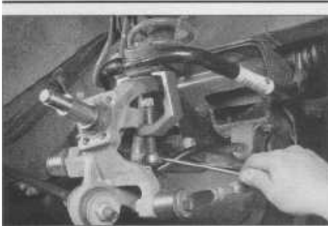
15.6 Use a puller to detach the upper control arm balljoint from the rear knuckle
