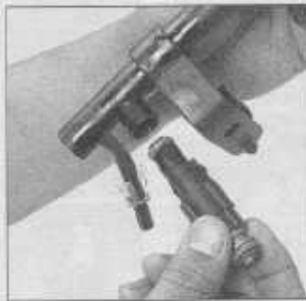
16.26b ... then withdraw the injector from the fuel rail
