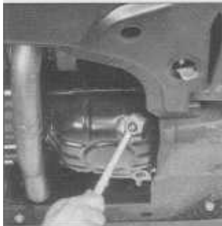
8.8 To avoid rounding off the corners, use the correct size box-end wrench or a socket to remove the engine oil drain plug
