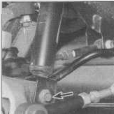
11.4 Remove the lower shock mount clevis bolt and nut (arrow)
