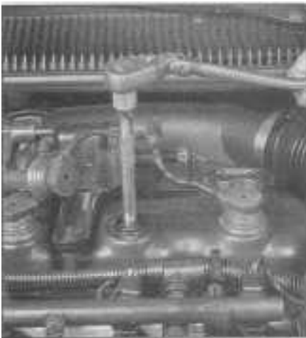
27.12 Use a ratchet and extension to remove the spark plugs
