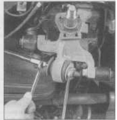
12.2 Use an open-end wrench to hold the trailing link from rotating while removing the nut and washer at the knuckle
