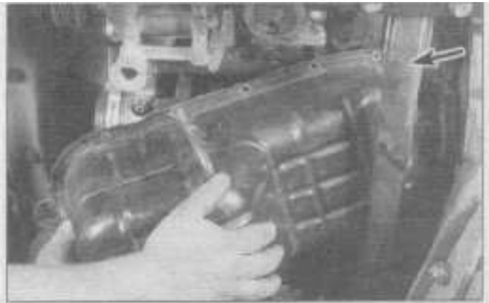
13.12 With the oil pump pick up tube removed, the oil pan can then be withdrawn over the engine support module (arrow)
