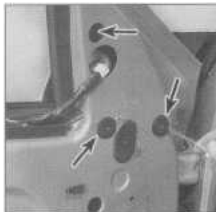
27.7 Pry off the caps from the exterior mirror mounting nut access holes (arrows)
