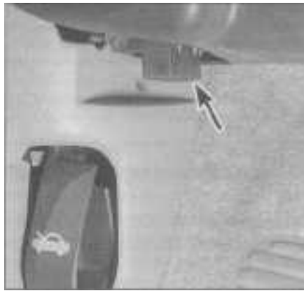
2.11 The OBD-II diagnostic connector (arrow) is located under the left (driver's) side of the instrument panel
