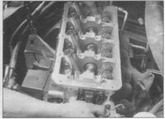
12.15a Carefully lift the cylinder head straight up and place the head on wood blocks to prevent damage to the sealing surfaces (2.0L engine shown)
