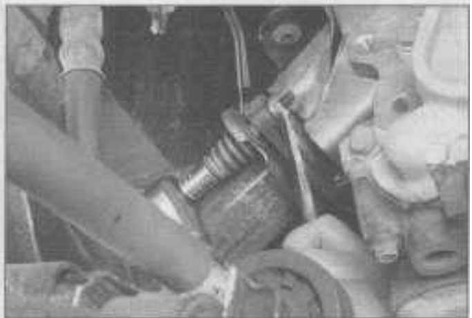
5.3 Using a box wrench on the nuts and a socket on the bolt, remove the shoulder bolts, springs and nuts securing the exhaust pipe to the exhaust manifold
