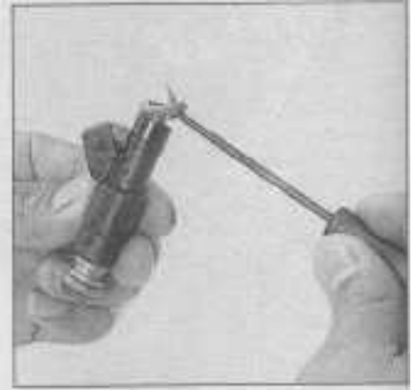
16.26c Remove the old O-ring seals from the fuel injector and discard them
