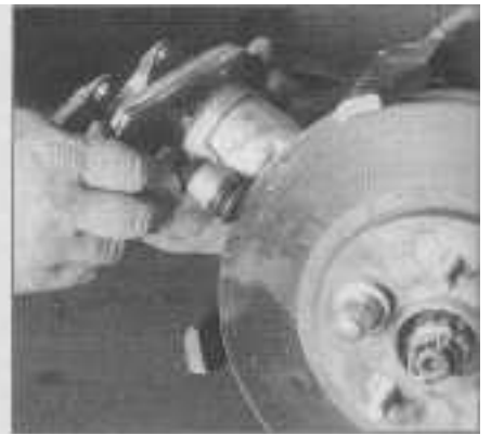
3.4i Install the inner brake pad - make sure the retaining spring is fully seated into the piston bore
