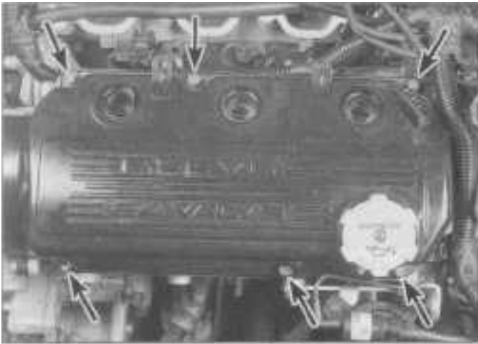
3.6 Valve cover mounting bolts (arrows)
