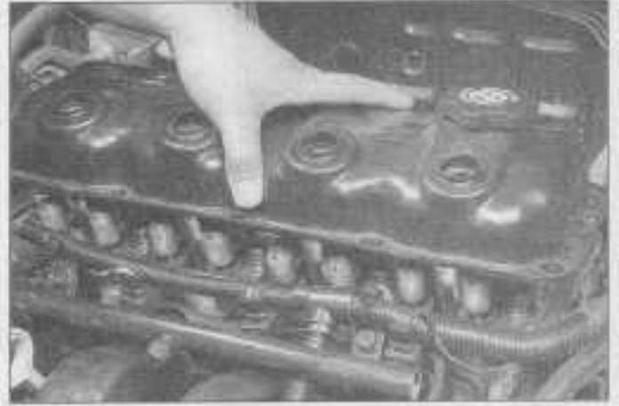
3.5b . . . and lift the cover and gasket off the cylinder head
