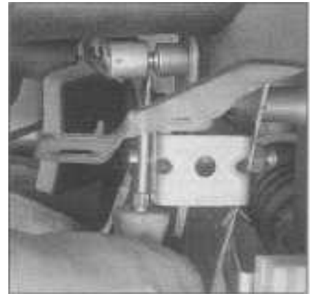
3.5b . . . next, wedge a narrow flat-blade screwdriver between the up-stop/spacer retainer and the clutch pedal pivot pin, then slide the up-stop/spacer off the pivot pin ..
