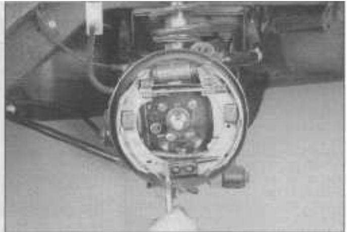
6.4a Using locking pliers, grasp the lower return spring and detach it from the leading brake shoe (left hand brake assembly shown)
