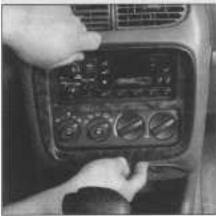
21.8 To remove the center bezel, simply pull it out evenly
