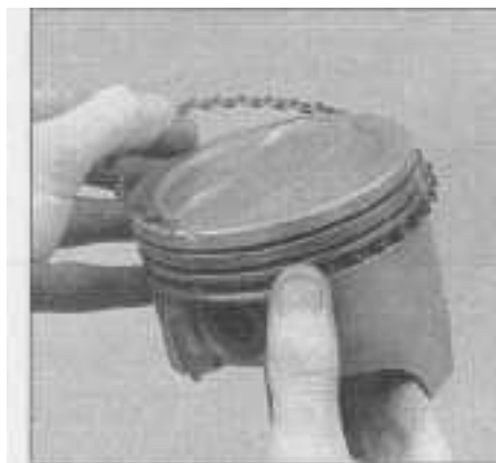
24.9a Installing the spacer/expander in the oil ring groove
