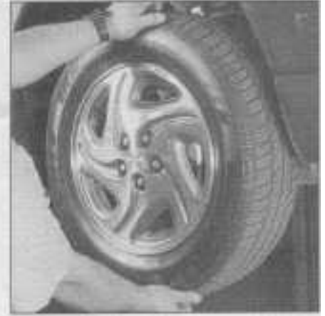
14.10 Checking the wheel bearing freeplay
