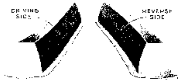
Figure 13—Heavy flank contact will result in noisy gears. Move pinion away from ring gear. Move gear in toward pinion if necessary to retain proper backlash.
