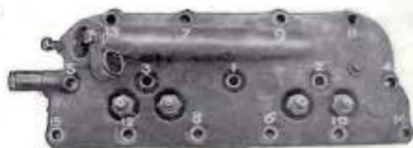
The order in which the cylinder head holding down nuts should be loosened and tightened up is as above.
