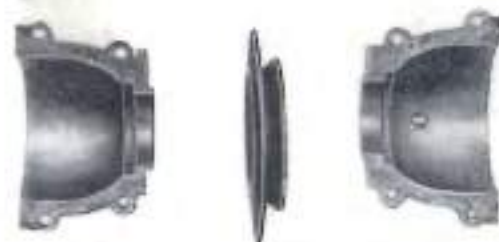
The two halves of the ball joint housing with ball joint locking ring.
