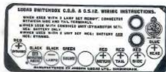
Fig. 7. Inside view of front cover plate of switchbox showing wiring instructions.
