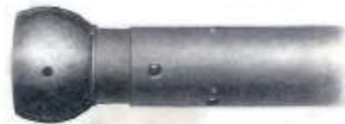
The torque tube ball joint which should be lubricated weekly via the Tealuminite nipple on top of the ball joint housing.
