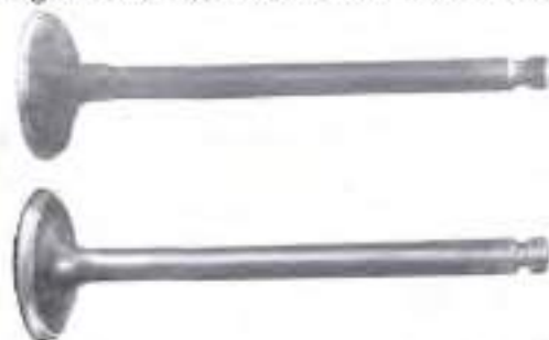
These two photographs show a valve before (top) and after grinding-in. Note the different appearance of their sealing faces.
