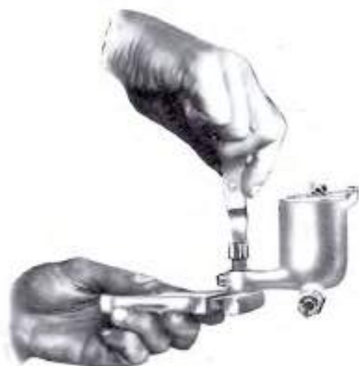
Removing the jet.
