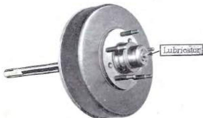
A lubricator is provided on the end of the axle shaft for lubricating the wheel hub.
