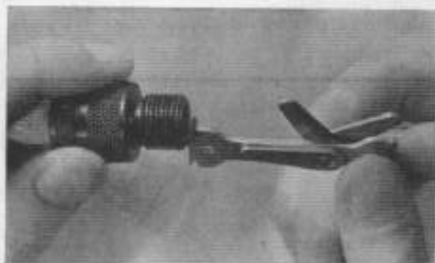
Adjustments should be made only by the side wire, and the combined setting tool and gap gauge illustrated can be obtained from the Champion Sparking Plug Co. or your Morris Dealer.
