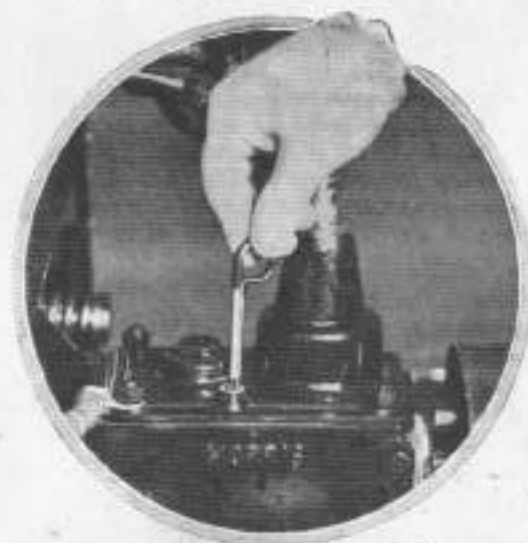
The rear end of the gearbox, showing the oil filler and some adjacent components.
