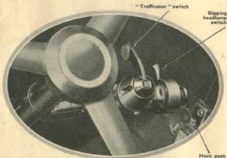
The "Trafficator" control on the steering column, and the combined horn button and dimming switch for the headlamps, which are conveniently situated close to the driver's right hand.
