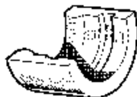
18G 705 G. Bearing Centre Race Remover Adaptor
