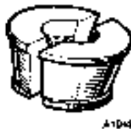
18G 264 D. Bevel Pinion Bearing Outer Race Remover Adaptor
