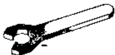
18G 313. Steering Tie-rod 'C' Spanner
