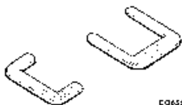
18G 1145. Rocker Type Switch and Bezel Remover
