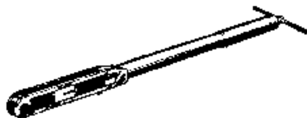
18G 372. Torque Wrench—30 to 140 lb. ft. (4.15 to 19.4 kg. m.)
