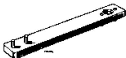
18G 312. Steering Tie-rod Pin Spanner
