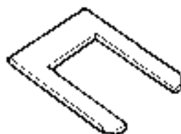
18G 1201. Rocker-type Switch (Slim Type) Remover
