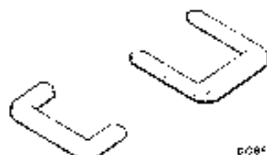
18G 1145. Rocker Type Switch and Bezel Remover.
