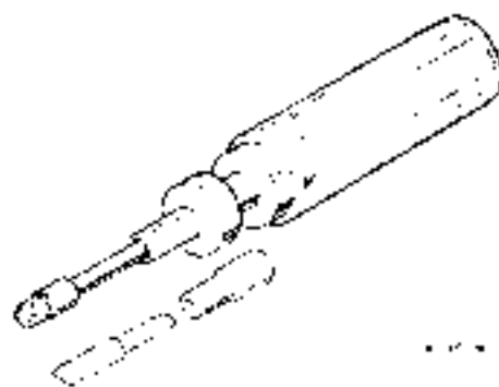
18G 681. Torque Screwdriver Set 0 to 40 lb. in. (0 to 400 gm. m.).
