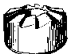
18G 174 D. Valve Seat Narrowing Cutter—Top (exhaust).
