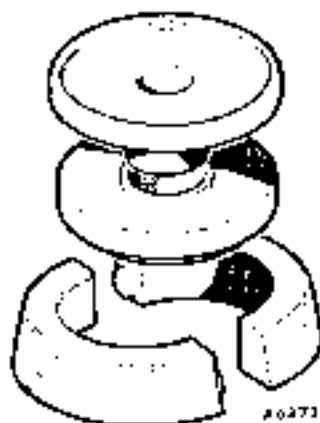
18G 47 AP. Annulus Tail Shaft Bearing Remover and Replacer Adaptor.
