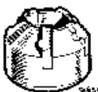
18G 28 A Valve Seat Glaze Breaker (inlet).
