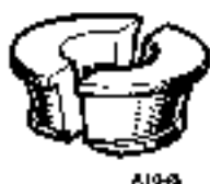
18G 264 AD. Bevel Pinion Outer Race Remover and Replacer Adaptor (Front).
