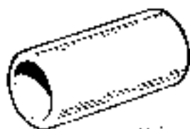
18G 183 A. Oil Pump Barrel Remover Adaptor.
