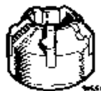
18G 25 A. Valve Seat Glaze Breaker (exhaust)
