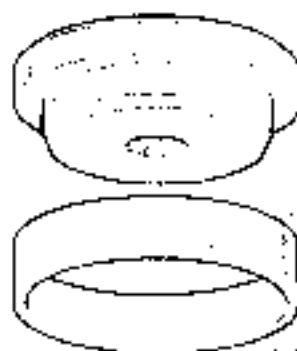
18G 134 CQ. Crankshaft Oil Seal Replacer Adaptor.
