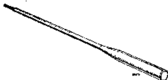
18G 471. Dummy Layshaft.
