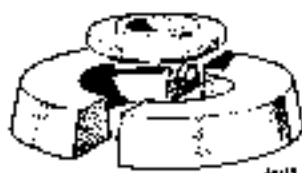
18G 47 AH Bevel Pinion Inner Race Remover and Replacer Adaptor.
