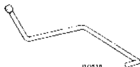
18G 1117. Pump Body Holder and Seat Remover.
