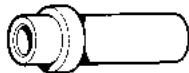
18G 1150. Basic Tool Remover and Replacer—Gudgeon Pin.
