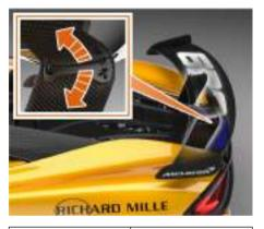
Rear wing adjustment 9 Nm (7 lb.ft) bolt torque figure
