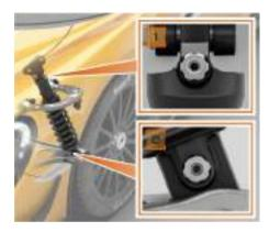
The rebound adjuster is located at the base of the damper body, rebound adjustment has 35 different positions. The adjustment wheel should be rotated clockwise to stiffen and counter clockwise to soften.
