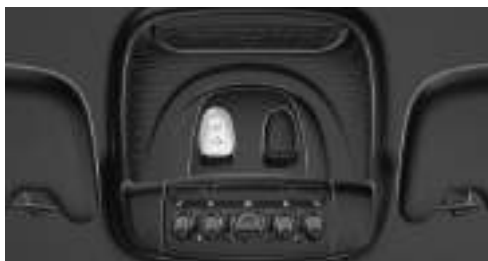
SOS button in the roofliner
