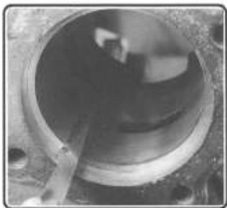
Figure 42. Measuring piston ring gap.
