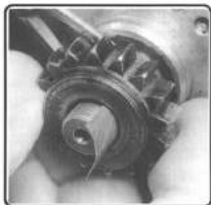
Figure 40. Sanding the output sprocket.
