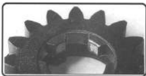
Figure 25. Modified sliding gear.
