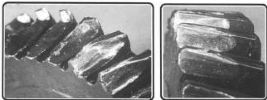
Figure 17. Completely ruined gear.
