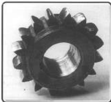
Figure 23. Scored driving sprocket.
