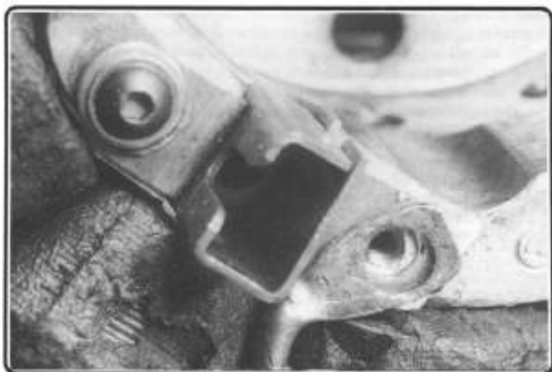
Figure 32. Brush-holder mounting screws and insulation.
