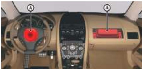
The front airbags (A) only deploy in a serious front collision.
