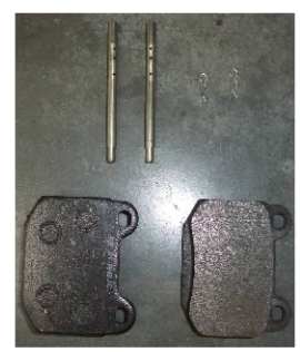
Pins, R-Clips and Pads Removed
