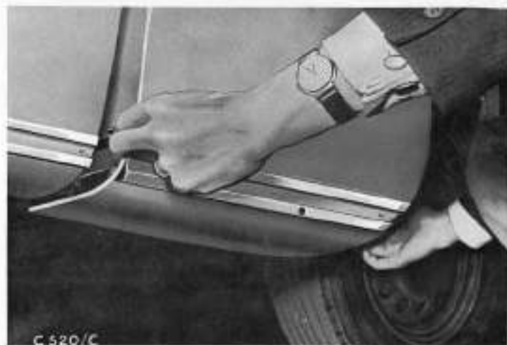
Fig.29 Opening the Wing Bay
