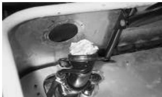
Figure 189: Old filler boss removed
