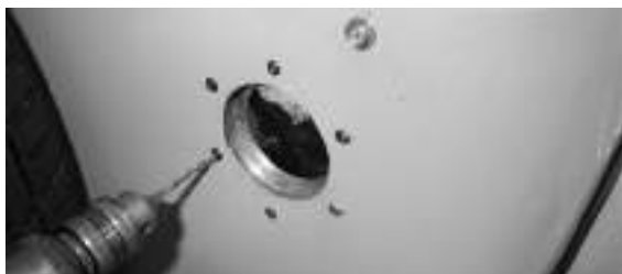
Figure 188: Drill out the six rivets
