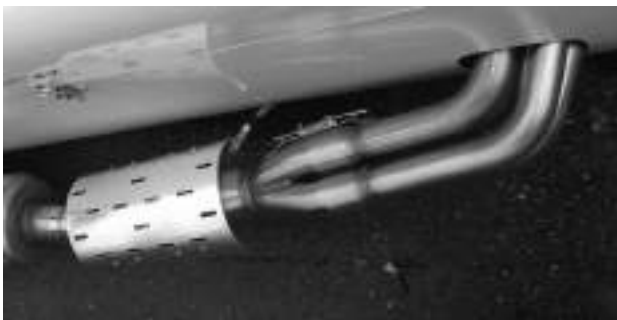
Figure 49: Primary pipes and collector/catalyst
