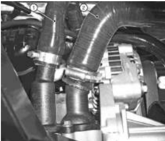
Figure 53: Bottom hose engine connection (viewed from bellow)
