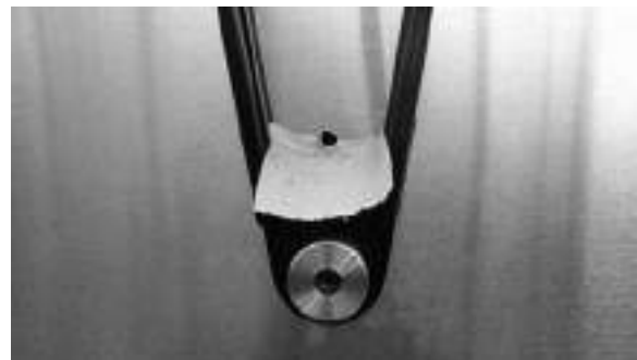
Figure 199: Drilled hole above spare wheel boss
