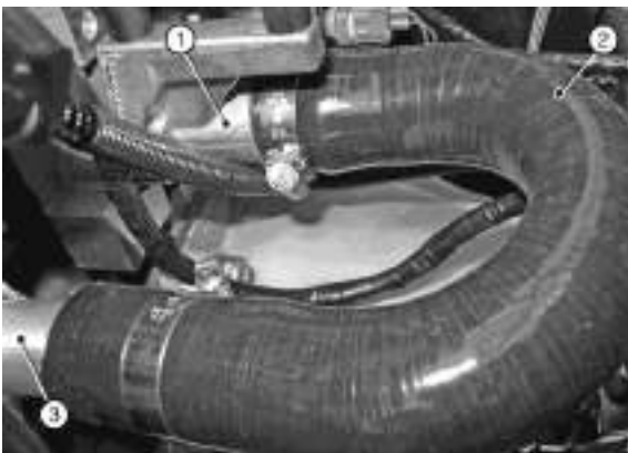
Figure 41: Water rail and 'U' hose
