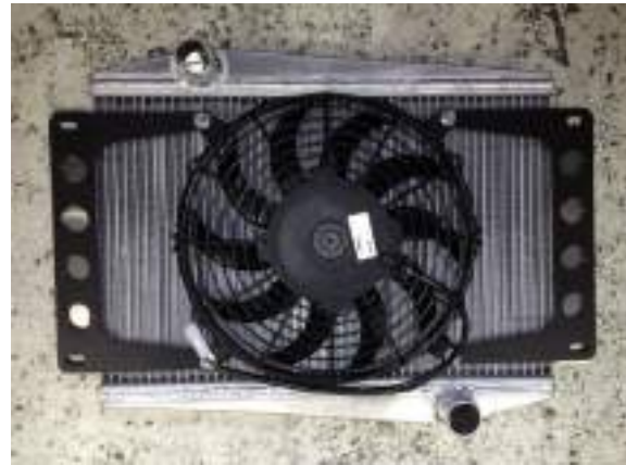
Figure 54: Radiator/fan prior to fitting
