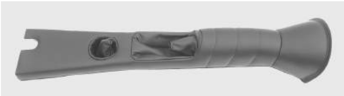
Figure 14: Transmission tunnel top
