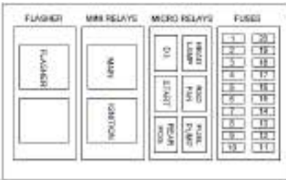
Figure 27: K6A Fuse box and relay layout
