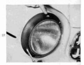
The adjustment of the headlamps is made on the adjustment screen or with an adjustment device. Load vehicle with 2 passengers or corresponding weight,
