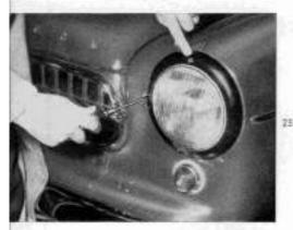
Separate lamp carrier by tipping of the tension clip from headlamp, remove headlamp.
