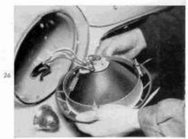
Caution: The adjustment of the "Hella" headlamps is also effectuated on the two screws top and L.H., seen from the front. The left screw (in figure with screwdriver) is for the side direction, the upper screw (in figure designated by finger) for the elevation of height.
