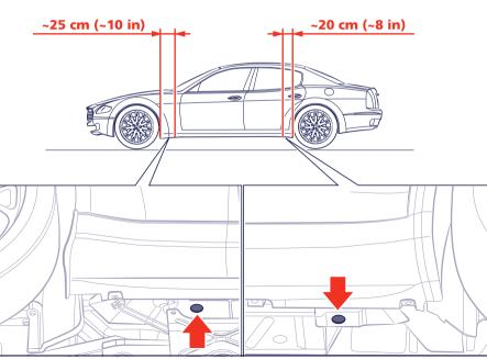
The jack can be used only to replace the wheels. Under no
