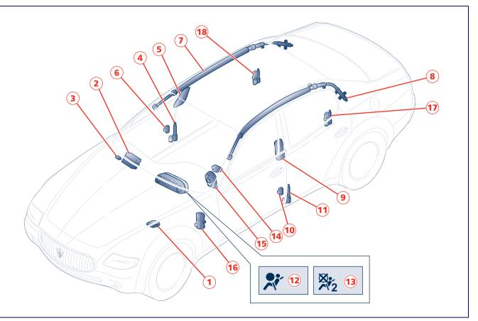
The vehicle is equipped with 6 airbags (2 front and 4 lateral ones) and electronically-operated pretensioners for all of the seat belts except the rear central one.
