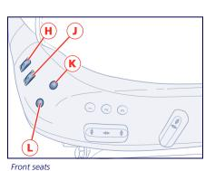
Also, using wheel button J the intensity of the heating can be set at 3 levels.
