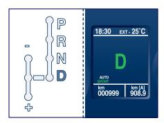
gearshift lever; it is disengaged by pressing the button and the brake pedal at the same time It is advisable to also hold the brake pedal depressed when moving the gearshift lever to the other positions.
