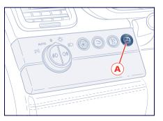
frequency increases as the vehicle approaches the obstacle. The acoustic signals are emitted by two buzzers, one under the dashboard (if the vehicle is equipped with front sensors) and one in proximity of the luggage shelf.
