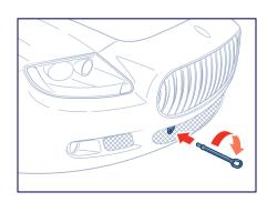
Tow the vehicle using the towing hook found in the toolkit. Screw the towing hook down tightly in its seat, on the lower, right-hand side of the front bumper.
