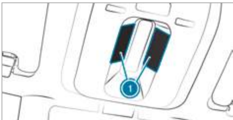
① Arrangement of the cameras of the front camera in the overhead control panel
