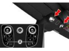
Press the **TRIP** button (A) for less than three seconds to cycle through the trip computer functions one at a time. Trip computer information is viewed in the message centre.
