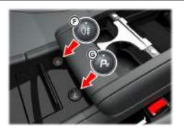
**[F] REAR FOG LAMPS:** Used with the dipped beam when fog or mist is causing restricted visibility. They **must** be set to OFF when visibility clears to reduce glare to the drivers of following vehicles.
