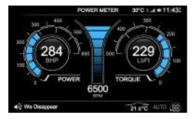
The screen will show both power and torque along with engine speed. On the power and torque dials there will be two readings: [1] LIVE VALUE: Instant values as read from the vehicle. Shown in selected infotainment display colour (Refer to 'Infotainment Personalisation', page 6.4)
