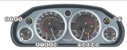
[1] LOW FUEL WARNING: Comes ON when only approximately 13 ltr of fuel or 80 km distance is available. At 13 ltr / 80 km and 7 ltr / 40 km an audible 'beep' will sound and the 'estimated distance' message will show (for 20 seconds) in the message centre. The arrow head shows which side of the vehicle the fuel flap is.
