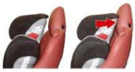
Motor the passenger seat fully to the rear and install the Britax 'Evolva 2-3 ISOFIT' child seat to the passenger seat ISOFIX bars as per the manufacturer's instructions. Adjust the height of the child seat headrest as required according to manufacturer's instructions. Tilt the passenger seat back forward until the top of the child seat comes into contact with the passenger seat as shown.
