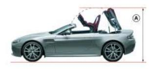
If the vehicle is moving while the roof is being raised or lowered, roof movement will continue, while the roof switch is pressed, until the roof has locked in the raised or lowered position.
