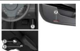
[1] : Front footwell lamps: Type: W5W (Blue). Rating: 5W. [2] : Door puddle lamps: Type: C5W (Festoon). Rating: 5W. [3] : Reading lamps: LED
