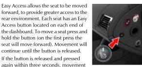
will continue in the same direction. If the button is released and pressed again after four seconds the seat will start to move in the opposite direction. When moving rearwards the seat will return to its original position while the button stays pressed.
