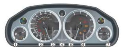
[1] FUEL GAUGE: Shows how much fuel is in the fuel tank. Refuel as soon as possible when the low fuel symbol comes ON.
