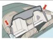
To remove the wind deflector pull up at the points shown to un-clip the two tabs from the top seat belt mounts. Remove the wind deflector from the vehicle, fold it flat, put it in the storage bag and place the bag in the storage area in the vehicle boot.
