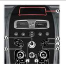
VOLUME/ON/OFF: Volume control. Press to mute the audio system. Press and hold to turn the infotainment screen on or off.
