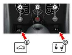
[A] DYNAMIC STABILITY CONTROL: The DSC system is always ON when the ignition is ON. Press and hold for four seconds for OFF. Press and release to set to ON.
