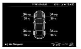
The tyre status screen is to be used as a visual support for the TPMS indicator in the message centre. If the tyre status screen is not selected in the infotainment screen and a tyre fault does occur, warnings will **only** appear in the message centre.
