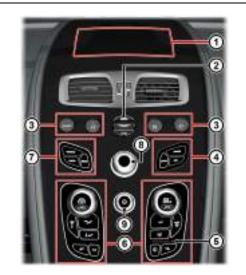
[1] **INFOTAINMENT SCREEN:** Opens when the infotainment system [9] ON/OFF/VOLUME: Press to switch the Infotainment system ON and OFF. Rotate to adjust the volume control. is set to ON.
