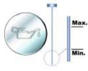
Approximately one litre is required to bring the level from Min. to Max.
