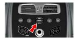
A Warning: Only use the vehicle key in the ignition control. Do not place any objects, including fingers, into the ignition control other than the vehicle key. Objects other than the vehicle key may cause the ignition control to fail.
