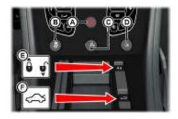
[A] HAZARD WARNING LAMP: Press to set the hazard warning lamps to ON or OFF.
