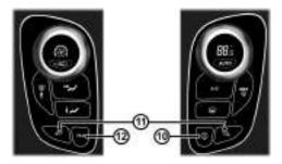
[10] (I) / READ: Press to view and acknowledge messages in the message centre (Refer to 'Instrument Cluster', page 4.3). [11] **READING LAMPS:** Driver and passenger reading lamps. [12] T1/T2: Select between the two trip meters in the message centre (Refer to 'Instrument Cluster', page 4.3).
