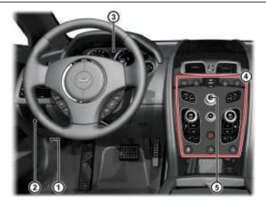
[1] FUEL FLAP RELEASE: Press to open the fuel flap. Close the fuel flap by pressing down on the flap until the lock engages.
