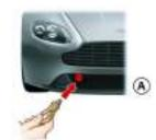
The towing eye has a left hand thread.
