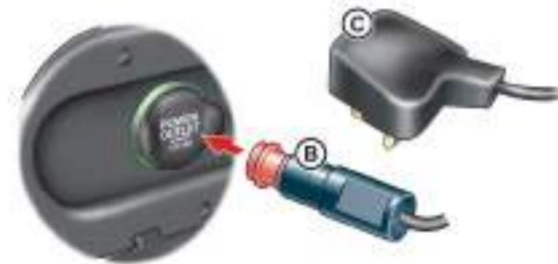
To remove the battery conditioner first disconnect from the mains supply, then from the vehicle socket.
