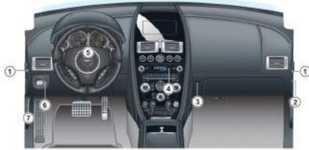
**[1] EASY ACCESS<sup>1</sup>**- Easy Access allows the seat to be moved forward, to provide greater access to the rear environment. Each seat has an Easy Access button located on each end of the dashboard. To move a seat press and hold the button (on the first press the seat will move forward). Movement will continue until the button is released (Refer to 'Easy Access', page 3.4).
