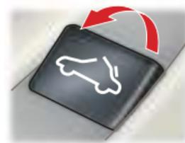
Push the Roof switch rearwards and hold until 'Roof Movement Complete' shows in the message centre (right).
