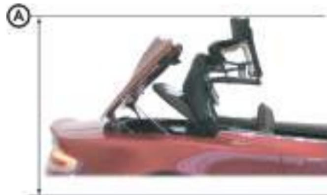
If the vehicle is moving while the Roof is being raised or lowered, Roof movement will continue, **while the Roof switch is pressed**, until the Roof has locked in the raised or lowered position.
