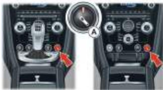
**Track Mode** - Press and release the ADS button (A) to start Track mode, which provides damping characteristics optimised for smooth, track conditions.
