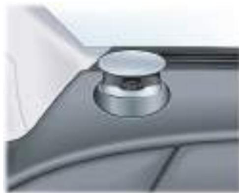
Two motorised acoustic lenses, mounted on either side of the dashboard, rise when the system is set to ON and stay raised until the Audio system is set to OFF.
