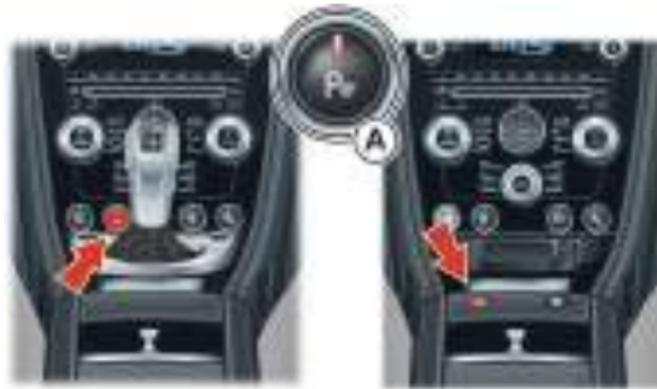
The Parking Assist button LED will come ON when the system is set to ON. The LED will flash if a fault is detected in the system.
