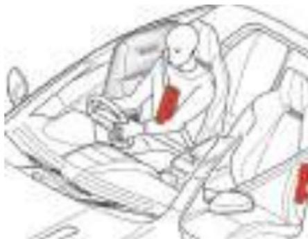
Do not change, modify or tamper with the steering wheel, passenger side fascia or any other part of the airbag system. Such actions could disable the system or cause inadvertent airbag deployment.
