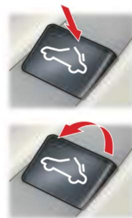
Release the switch and push again to change direction.
