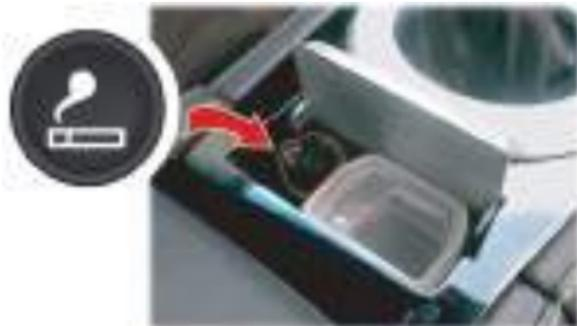
Remove the ashtray by opening the lid and pulling the glass tray upwards. Install the tray by placing it into position and push down.
