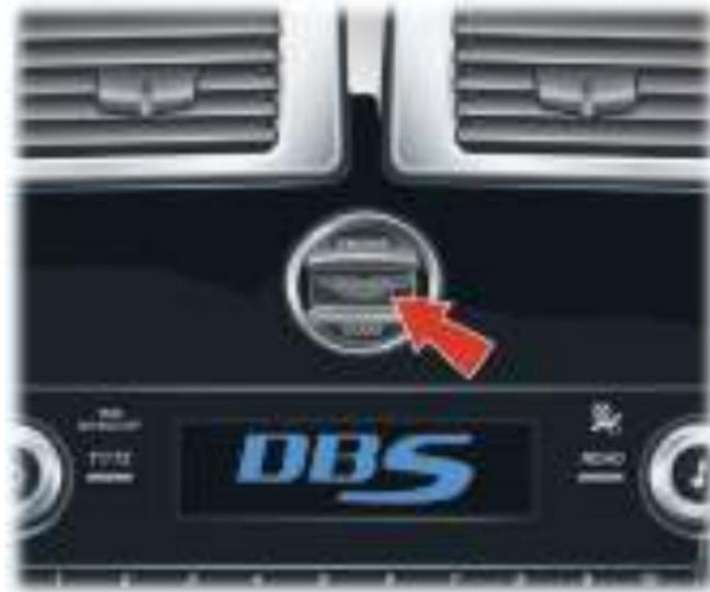
**Warning:** Only use the vehicle key in the Ignition Control. Do not place any objects, including fingers, into the Ignition Control other than the vehicle key. Objects other than the vehicle key may cause the Ignition Control to fail.
