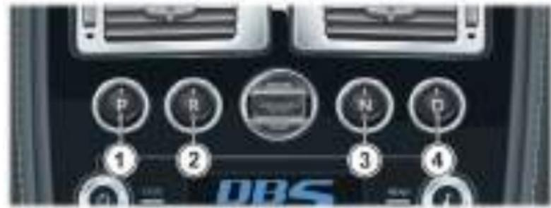
**[1] PARK-** Press and release to select Park once the vehicle is stationary. The transmission will mechanically lock. If the vehicle key is moved to position '0' or removed from the Ignition Control while the vehicle is at a standstill, the transmission will automatically select Park.
