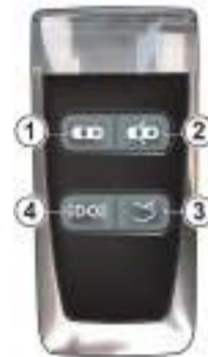
**[2] UNLOCK-** Press once for one step vehicle unlocking (Refer to 'Unlocking and Opening', page 2.6). The seats and door rear view mirrors move to their memorised positions (Refer to 'Seat Memory Function', page 3.7).
