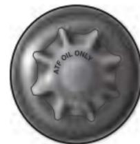
1. Remove the reservoir cap and wipe the dipstick clean with a lint free cloth. Replace and remove again. The fluid level should read between the Min. and Max. marks.
