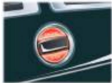
The vehicle key will sit flush with the Ignition Control bezel while the engine is running. The Ignition Control will show a white light when the engine is running, and then fade out.
