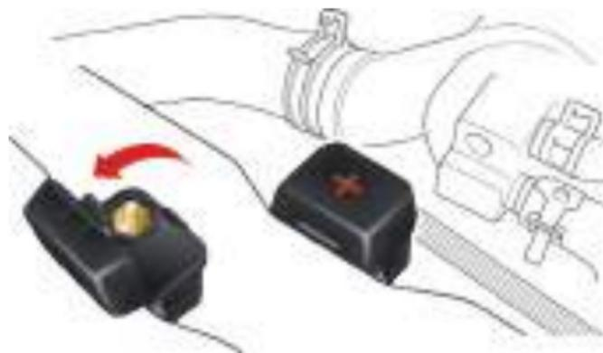
4. Connect the '-ve' (black) cable between the '-ve' (black) terminal of the donor battery and a good earth (-ve) point in the recipient engine bay (i.e. alternator mounting bracket).
