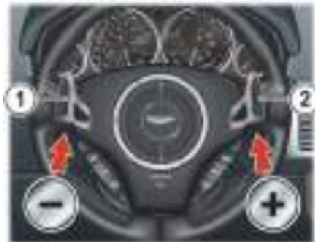
From park, reverse or neutral, and with the footbrake applied, pull back on either the upshift or downshift gearshift paddle to enter touchtronic mode. As the vehicle speed increases and decreases, make upshifts and downshifts by pulling and releasing the upshift or downshift gearshift paddle.
