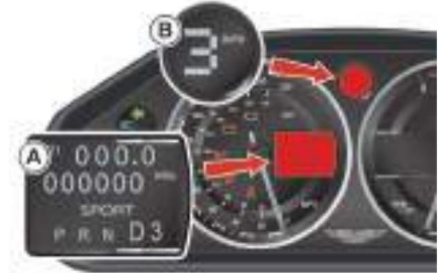
**📖** *If the vehicle speed is less than 4 km/h (2.5 mph), Reverse may be selected from Drive, without pressing the brake pedal, to enable a vehicle 'rocking' i.e. to enable vehicle movement out of mud, snow, etc. If 4 km/h (2.5 mph) is exceeded then the transmission will automatically select Neutral.*
