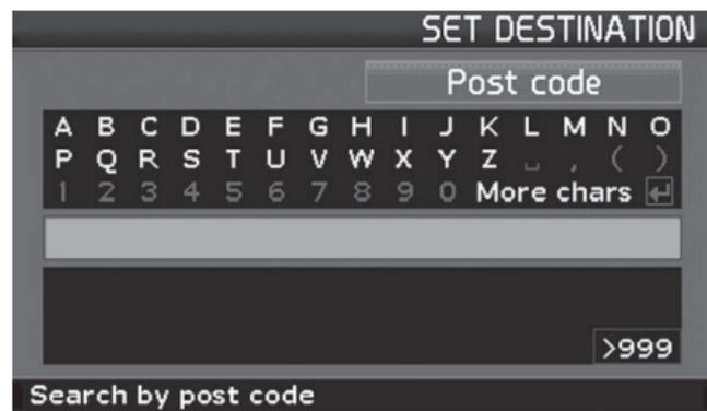
Use the **JOYSTICK** to select the desired letters and numbers from the character table and press **ENTER**. Move down and select a Post Code from the list. Press **ENTER**.
