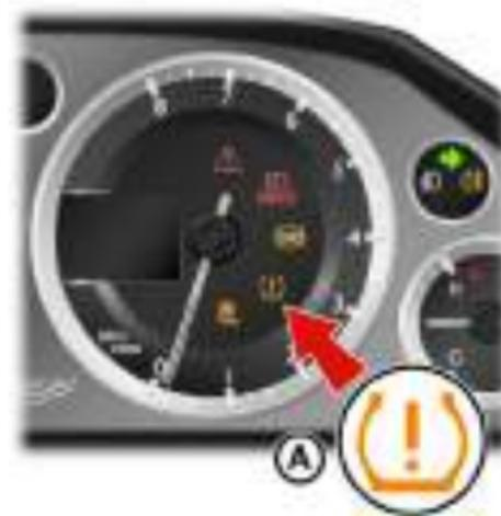
When the malfunction telltale is ON, the system may not be able to detect or send tyre pressure as intended. TPMS malfunctions can occur for a variety of reasons, including the installation of replacement or alternate tyres or wheels on the vehicle that prevent the TPMS from operating correctly.
