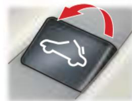
When lowering the window push the Roof switch forwards and release for 'One touch' operation.
