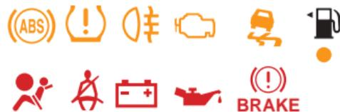
Under normal circumstances most warning symbols will go OFF at the end of the individual system check if system checks are satisfactory.
