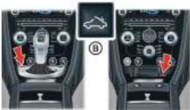
To raise or lower the rear quarter windows push and hold the Roof switch (B):
