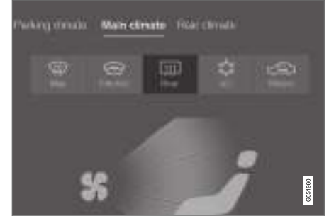
The button for heated rear window and door mirrors in the climate view.
